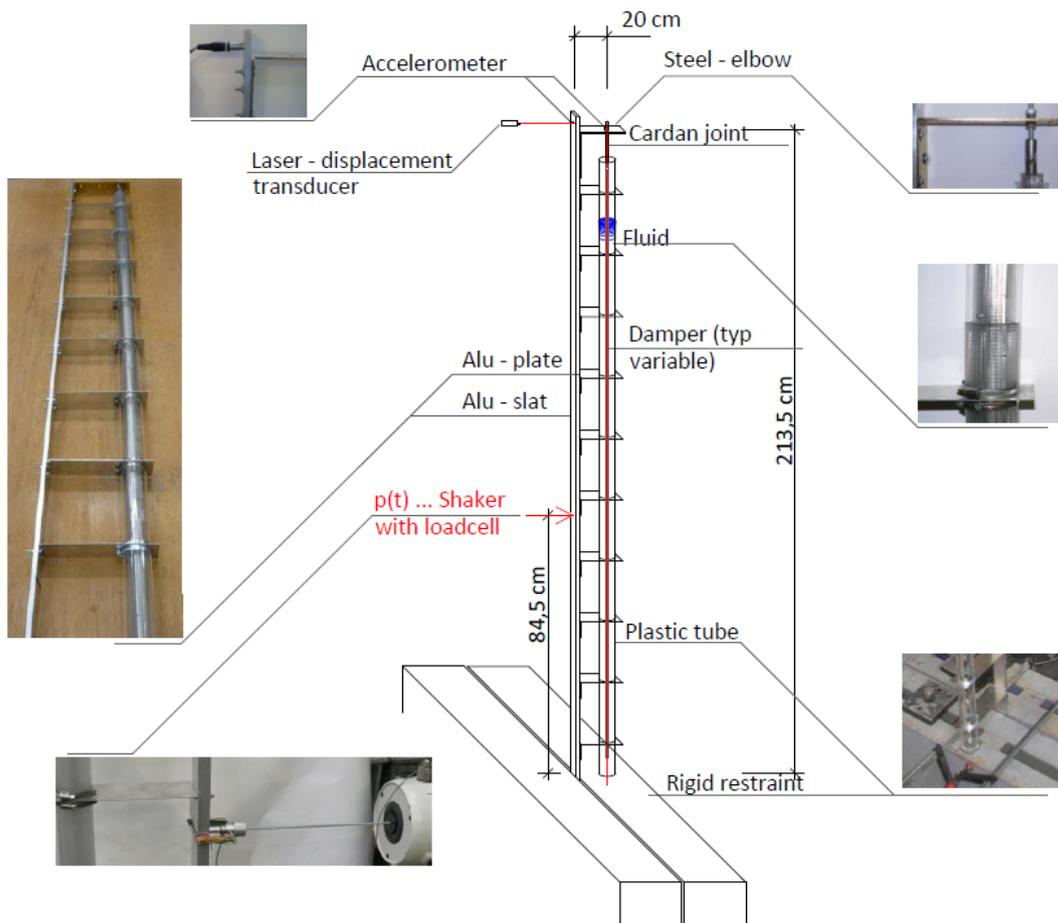
Figure 2. Experimental construction to test the new damping system (Neubauer, 2009)
