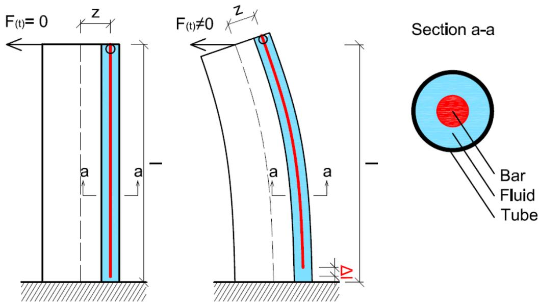
Figure 1. Cantilever beam with an integrated damper (Kollegger, 2009)
