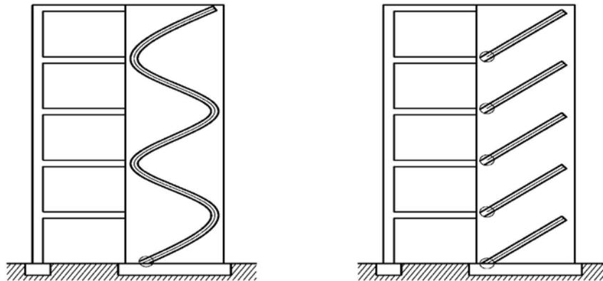
Figure 6. Damping system for shear deformation (Kollegger, 2009)
