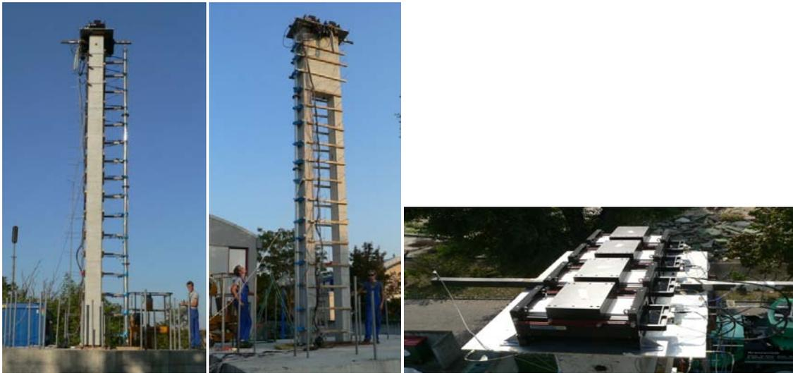
Figure 4. (a) and (b) bridge pillar with implemented damping system; (c) electro dynamic force generator
