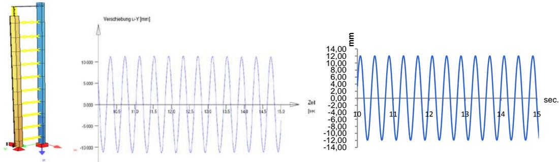
Figure 5. (a) Numerical model; (b) time- displacement results from FEM; (c) time- displacement results from laboratory tests
