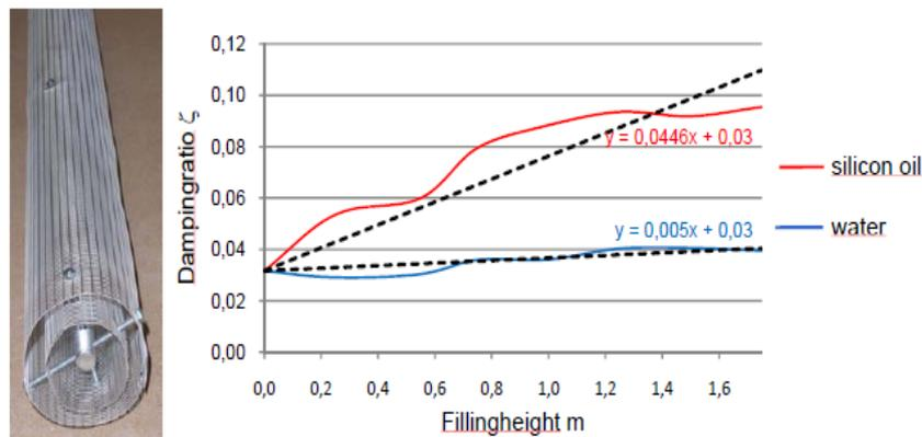
Figure 3. (a) Bar surrounded with perforated steel plates; (b) Diagram of the damping ratio (Neubauer, 2009)
