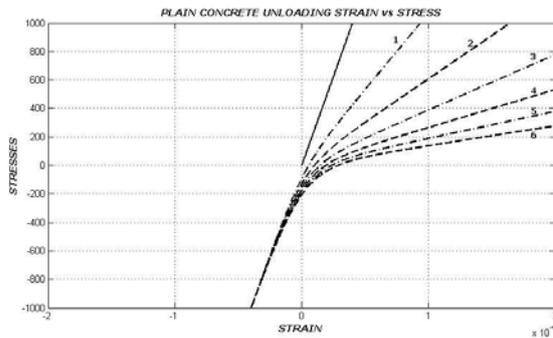
Figure 4. Stress vs. Strain curve for cyclic loading for different degradation level
