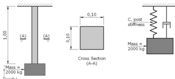
Figure 2. Concrete post used in the numerical study, (a) Concrete post's geometric dimensions, (b) Single degree of freedom model represents the concrete post model
