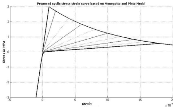
Figure 3. Stress vs. Strain relationship for both monotonic and cyclic loading
