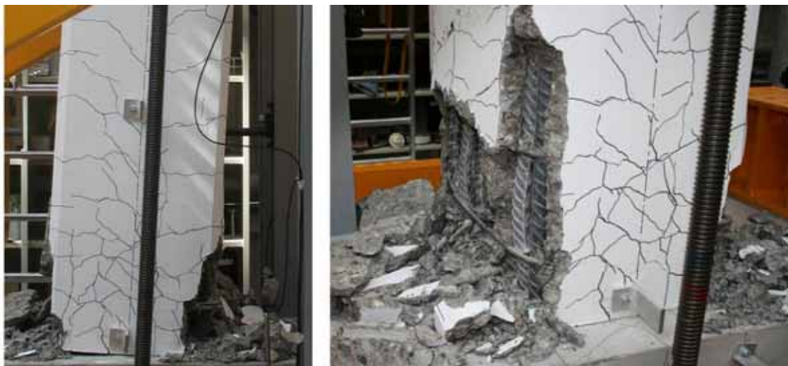
Fig. 10: Confined section of column P0 with buckling of rebars
