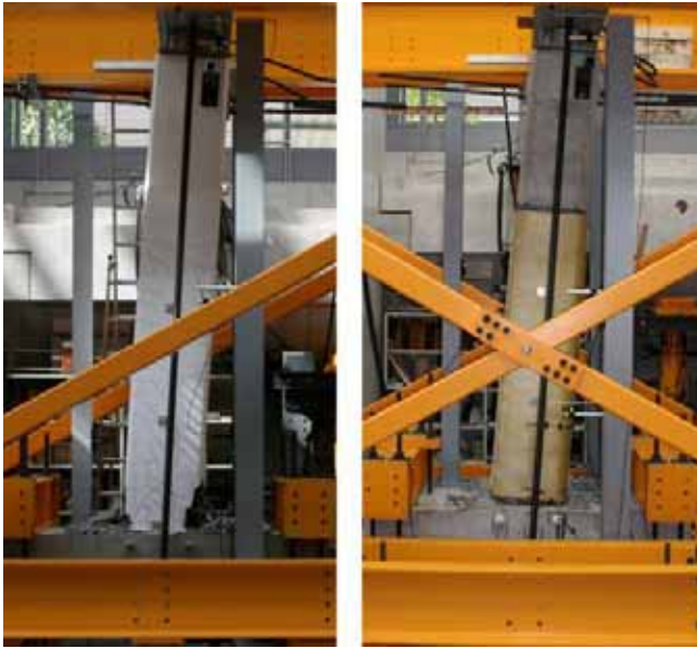
Fig. 9: Deformation at ruin of columns P0 & P1
