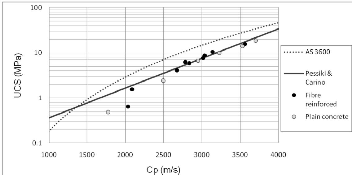
Figure 4 – Distribution of velocity vs. average compressive strength between 10 and 48 hours, plus empirical relationships by Pessiki and Carino (1988) and derived from (AS3600-2009).
