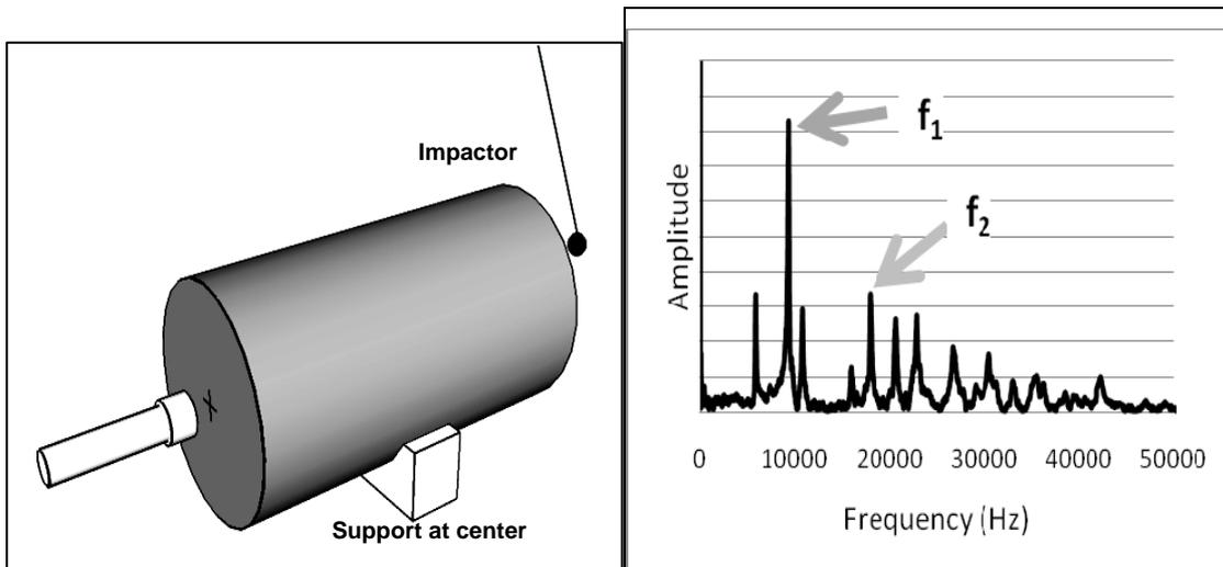
Figure 2 – Cylinder setup for longitudinal resonance testing as per ASTM C215
