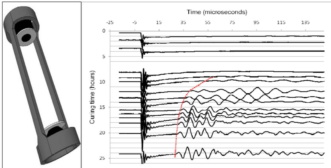
Figure 1 – Schematic depiction of the implanted sensor element (Left) and example ultrasonic dataset at different curing times, showing the onset of hydration at approximately 9 hours (Right), and subsequent reduction in first arrival times.
