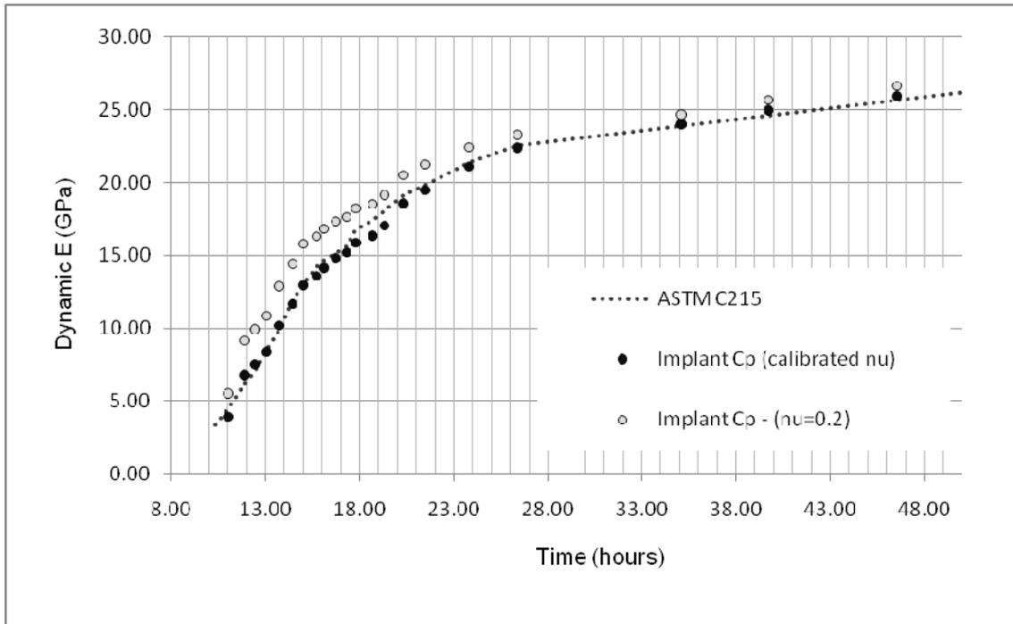
Figure 3 – Progression of dynamic elastic modulus as determined by harmonic cylinder resonance (line), and embedded P-wave velocity using measured and assumed values of Poisson’s ratio (dots).
