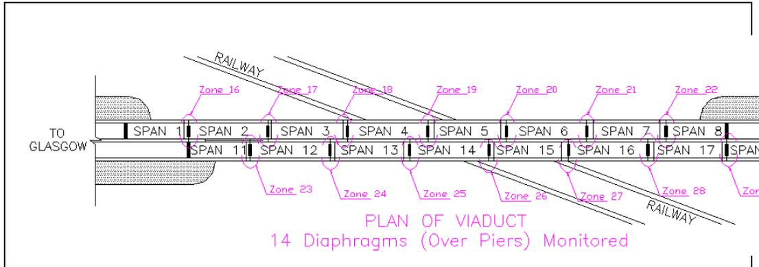
Figure 7: Overall acoustic monitoring plan for entire viaduct
