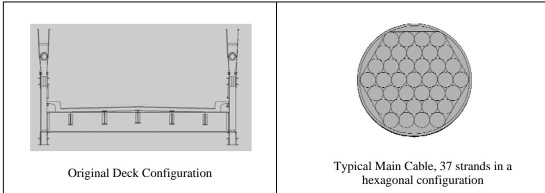
Figure 4: Typical Details of the Deck and Main Cable
