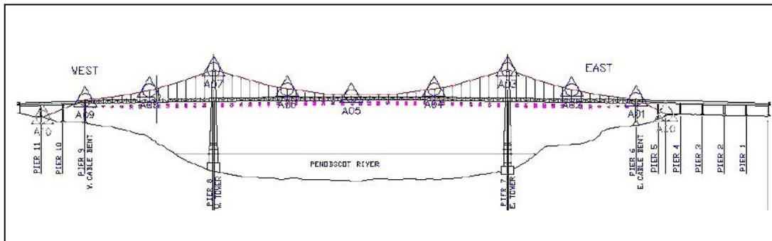
Figure 3: Waldo Hancock Bridge – Typical Cable Sensor Layout
