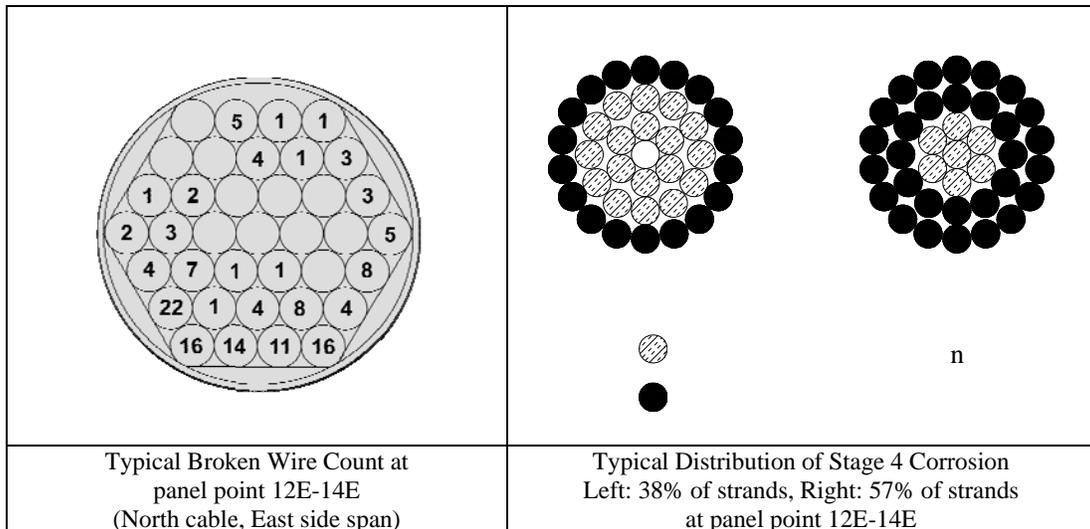
Figure 5: Typical Damage found. [Stages of corrosion are according to the Federal Highways Administration (USA) guidelines. A 4 stage system is used with stage 4 representing the most advanced stage of corrosion.]
