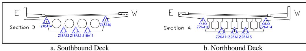
Figure 6: Cross-section of bridge showing acoustic sensor layout at each monitored location
