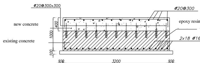
Fig 6. Detail of retrofitting foundation
