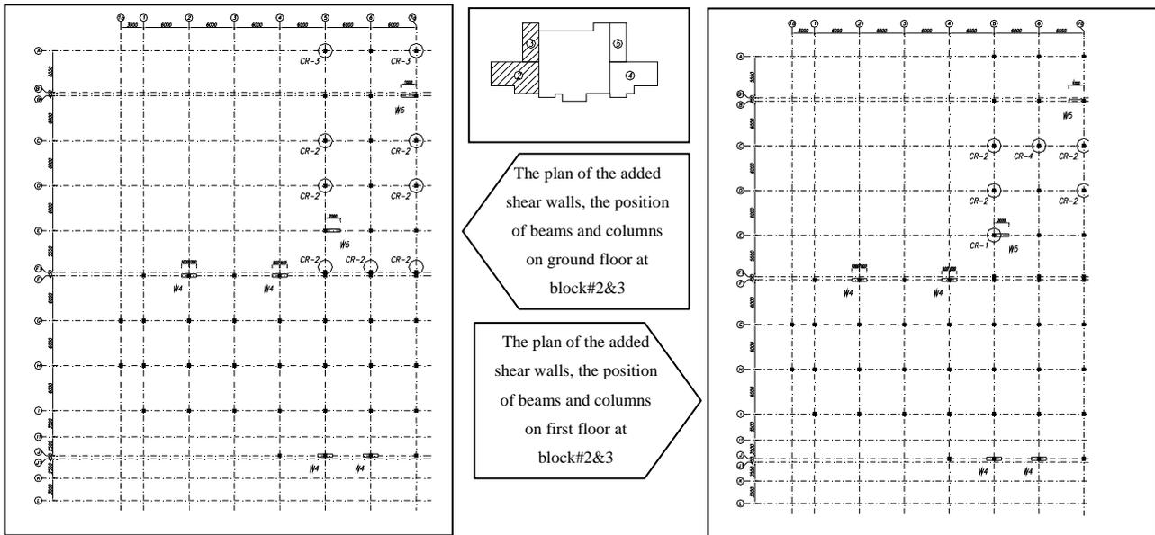
Fig 4. Location plan of Retrofitting shear wall, column, beams at block 2,3
