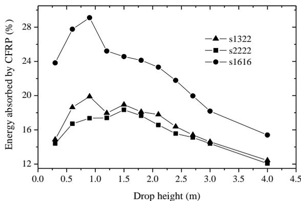
Figure 4. Drop height versus percentage of energy absorbed by the CFRP.
