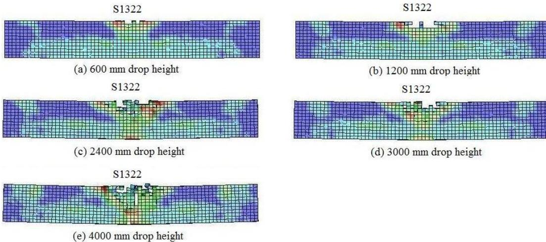
Figure 6. Crack patterns of CFRP-strengthened S1322 RC beam.
