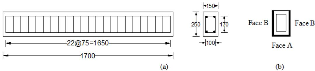
Figure 1. FEA validated models of beams (a) geometry and reinforcement details; (b) CFRP reinforcement layout (mm).
