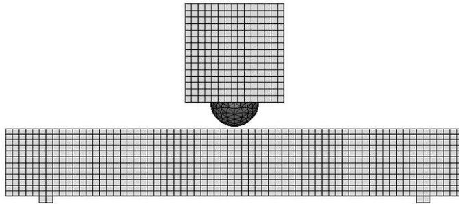
Figure 2. FEA mesh of reinforced concrete beam and impacting hammer.
