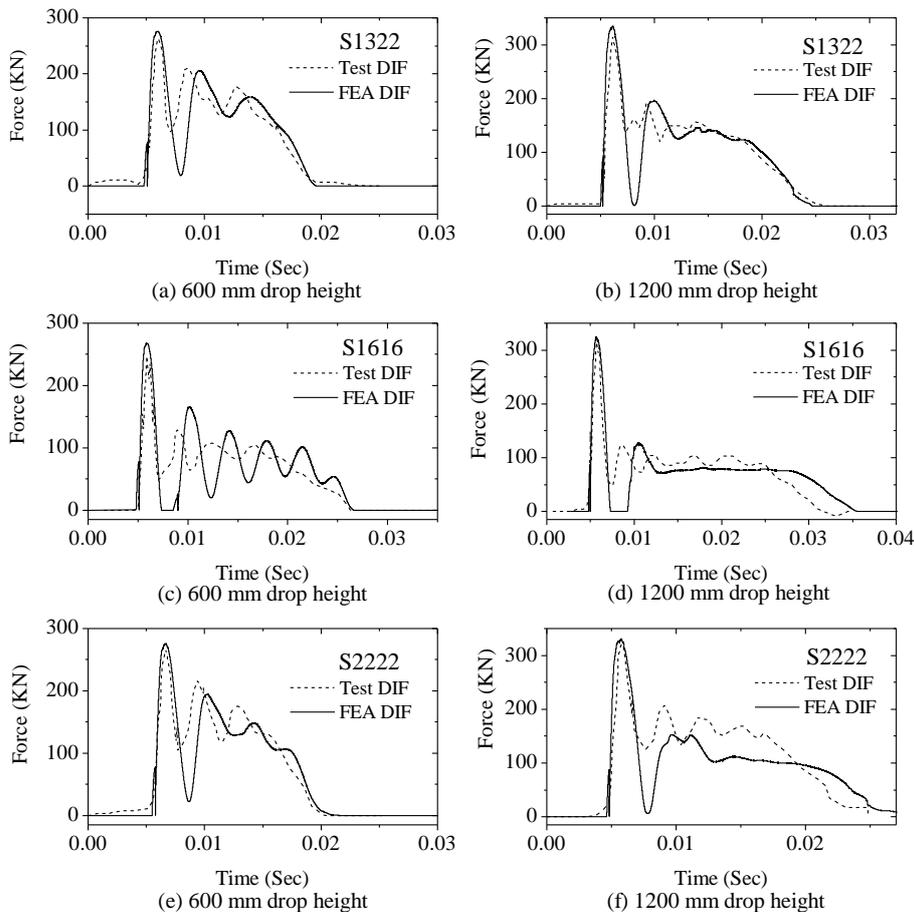
Figure 3. Dynamic impact force versus time history of the reinforced concrete beams
