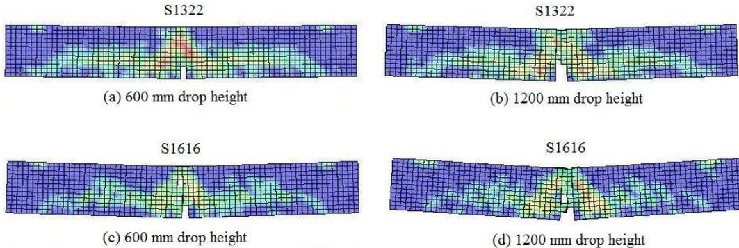
Figure 5. Crack patterns of as-built S1322 and S1616 RC beams.
