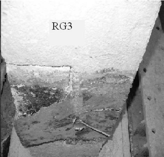
Figure 4. Debonding failure pattern of the strengthened Push-off specimen RG3.
