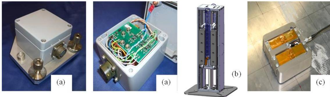
Figure 2. (a) New PZT fibre sensor; (b) Active absorber; (c) new concept of acoustical mass actuator
