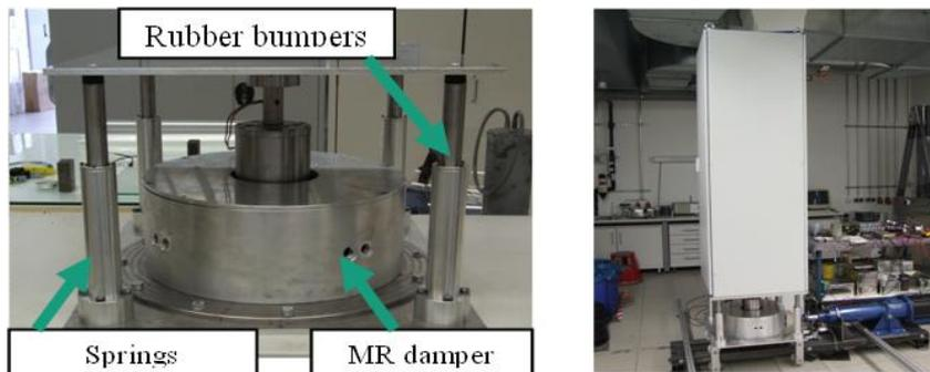
Figure 3. Semi-active system–MR damper for seismic protection and electrical control cabinet
