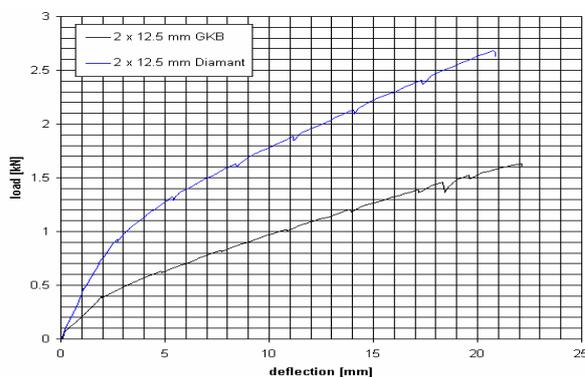
Figure 1. Bowing of “Diamant” boards compared to standard wall W 112 on CW 50 profiles (d=625 mm)
