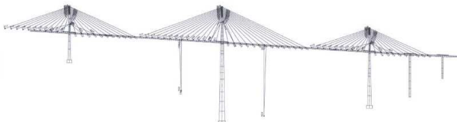
Fig 4 : structural model for the assessment of the residual bearing capacity of Mezcala
