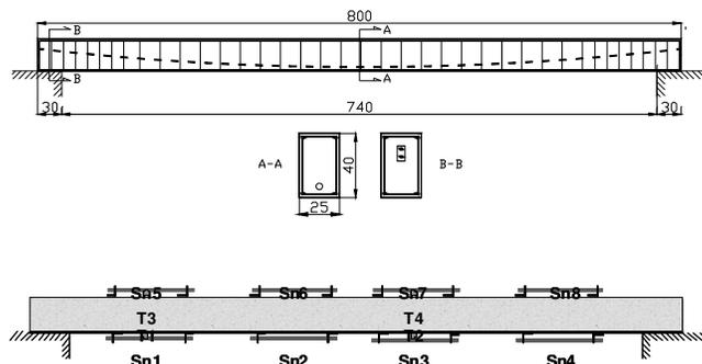
Figure 5. Specimen characteristics and sensor locations
