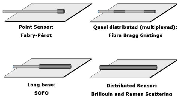
Figure 2: Fiber Optic Sensor Types
