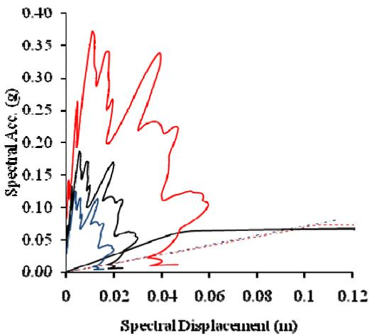
(b) Capacity and demand curves for Kjm000 earthquake (medium frequency content)
