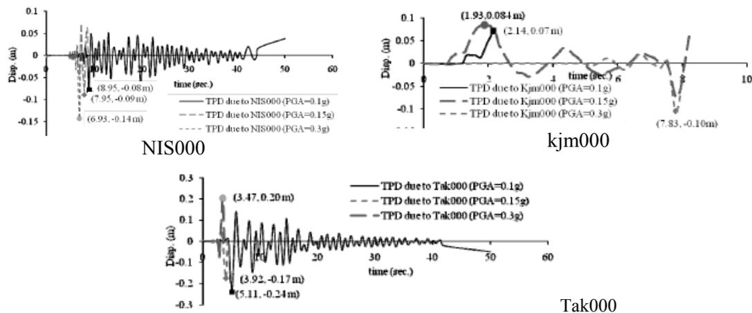
Figure 6. Top point Displacement due to different earthquake hazards
