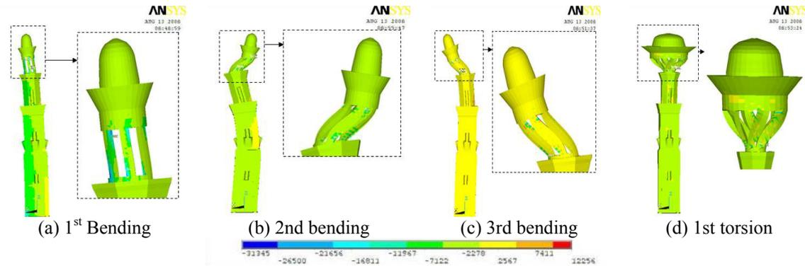
Figure 2. Stress Distribution in Different Mode Shapes
