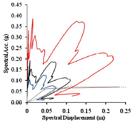
(c) Capacity and demand curves for Tak000 earthquake (low frequency content)
