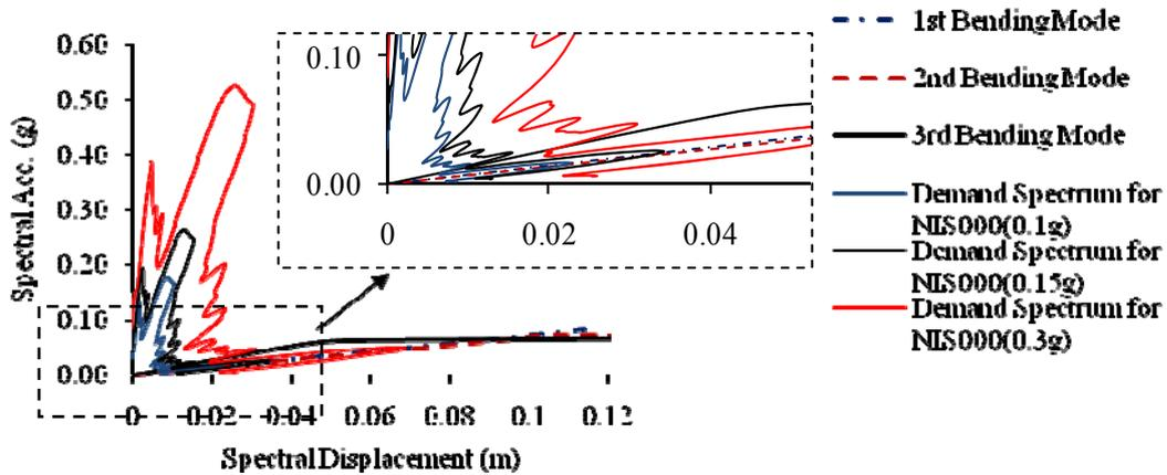
(a) Capacity and demand curves for NIS000 earthquake (high frequency content)
