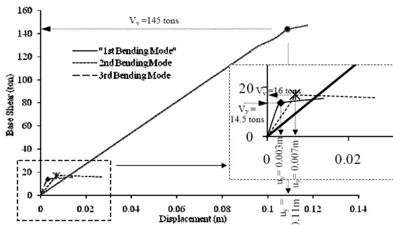
Figure 3. Base shear versus top point displacement due to pushover analysis
