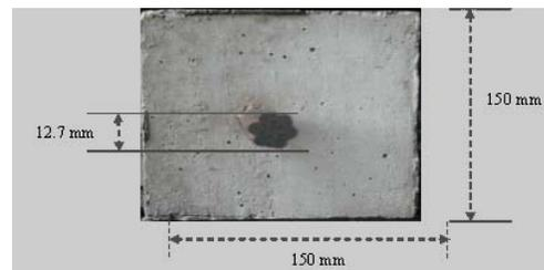
Fig. 3b: Cross-sections of beam with pre-stressing tendon
