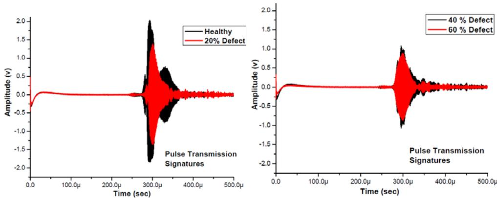
Fig. 5: Pulse Transmission signatures (Notch at L/2)
