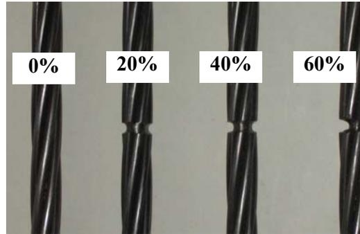
Fig. 2: Strands with 0%, 20%, 40% and 60% diameter reduction
