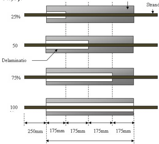
Fig. 3a: Strands in beams representing different extents of delamination
