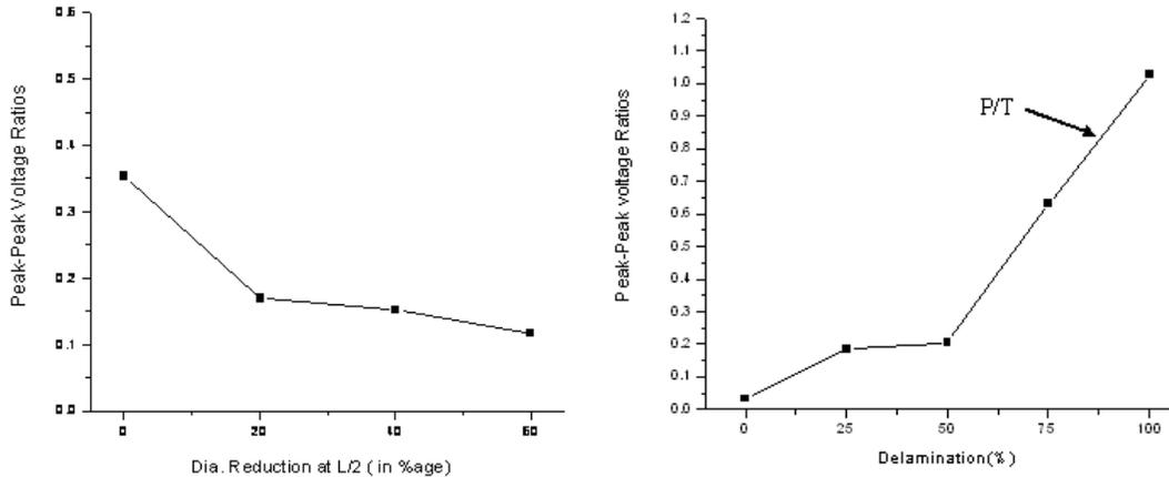
**(a) Peak to peak voltage ratio trends of P/T with notched specimens**
