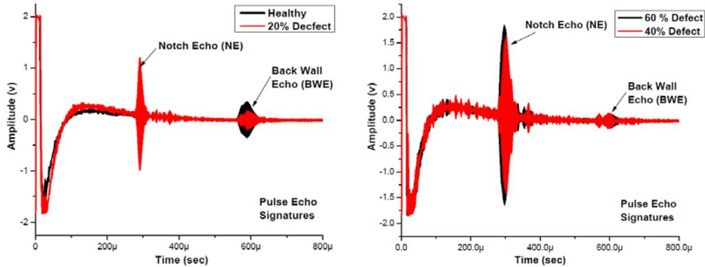
Fig. 4: Pulse Echo signatures (Notch at L/2)
