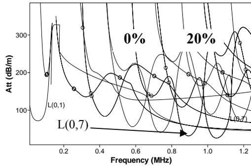
Fig.1: Attenuation dispersion curve for 12.7 mm tendon embedded in grout
