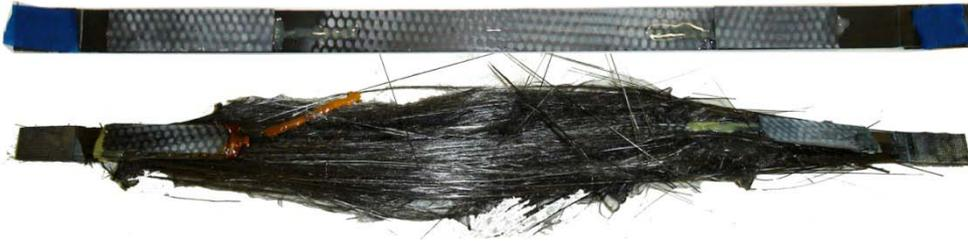
Figure 5 CFRP specimen 2.1, transient test, before and after the test.
