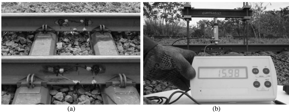
Figure 3. Special arrangement of strain gages for measure of wheel loads (a) and his calibration (b).
