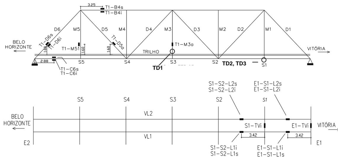
Figure 6. Location of some strain and displacement sensors installed on the bridge.
