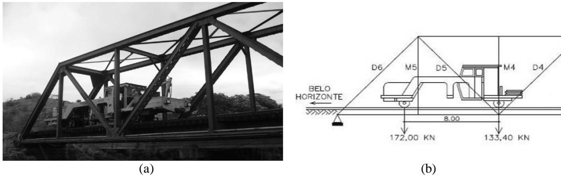
Figure 4. Plasser machine in the bridge during monitoring operations, with front axle on the vertical M4 (a) and his correspondent scheme (b).
