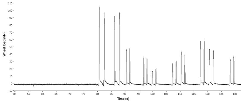
Figure 9. Wheel loads measured during passage of the Viliato train at a speed of 5km/h. The first load obtained ( $t \approx 80$  s) refers to the first axle of the locomotive.
