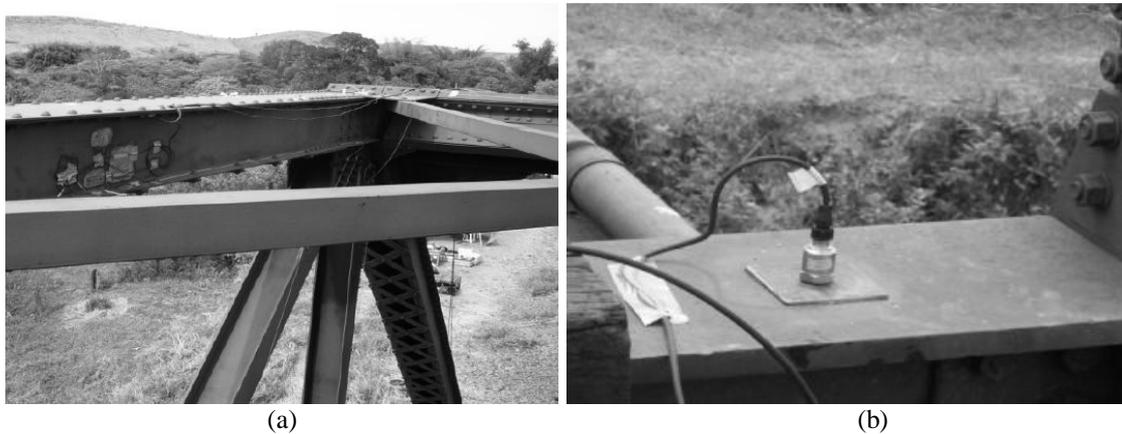
Figure 2. Strain gages and fiber optic sensors installed in the top chord (a) and accelerometer in the transverse floor beams.
