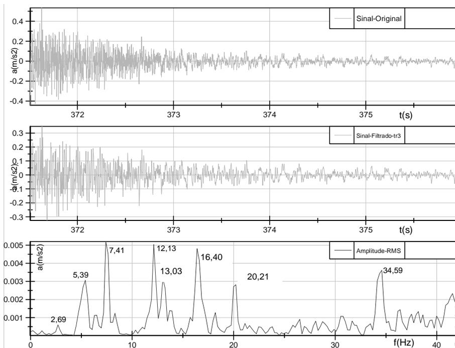
Figure 11. Free vibration response obtained in a transverse floor beam of the bridge.
