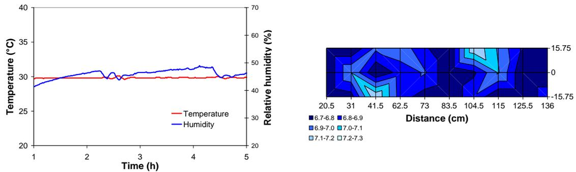
Figure 4. Temperature and relative humidity measurements during a typical test (left) and wind velocity measured at the surface of the concrete in the plastic shrinkage molds (right).
