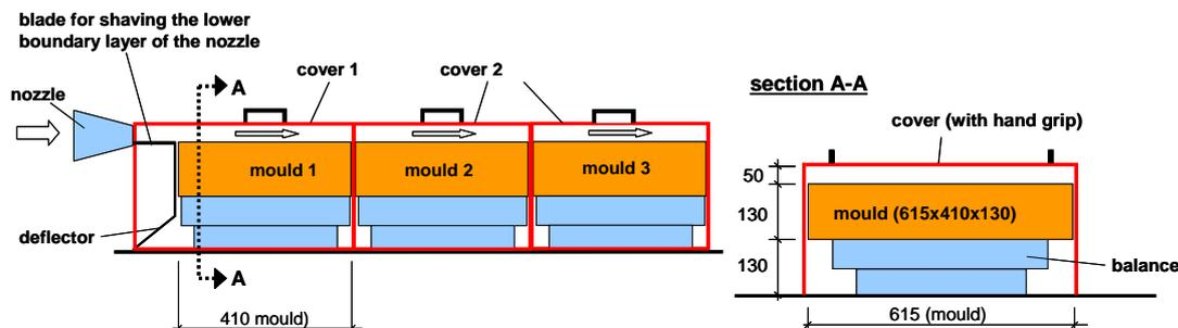
Figure 3. Schematic view of the setup for studying plastic shrinkage cracking of concrete mixtures.
