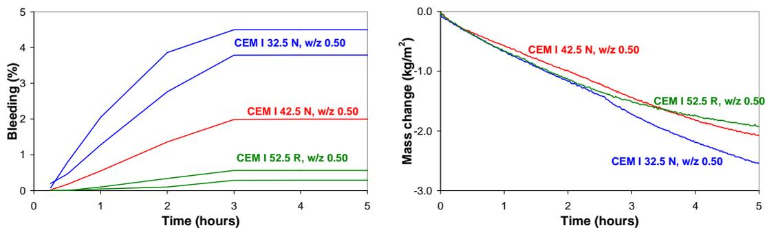
Figure 6. Bleeding (left) and mass change due to evaporation (right) of concrete mixtures with w/c 0.5 differing in the cement fineness.
