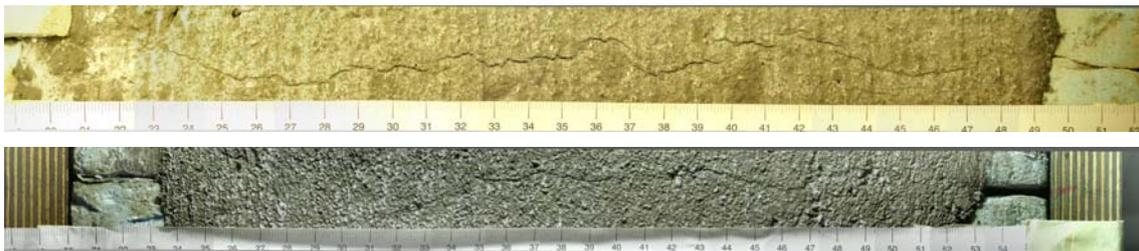
Figure 8: Example of plastic shrinkage cracks in concrete with CEM I 42.5 N (above) and in concrete with CEM I 52.5 R (below).
