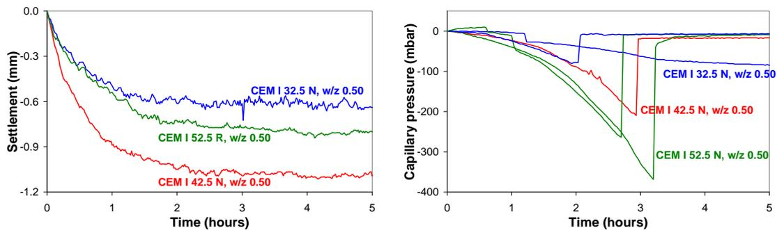
Figure 7. Settlement (left) and capillary pressure (right) of concrete mixtures with w/c 0.5 differing in the cement fineness.
