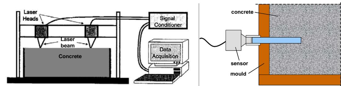
Figure 5. Schematic of settlement measurements by non-contact lasers (left) and of pore pressure measurements by tensiometers (right).
