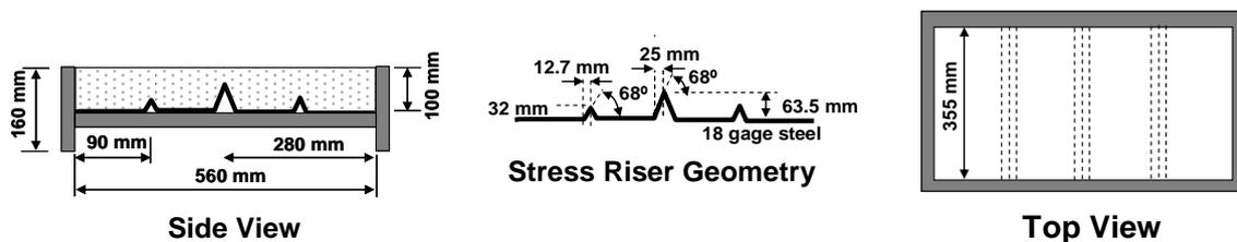
Figure 2. Moulds for measurements of plastic shrinkage cracking according to ASTM C1579-06 (from Lura et al. (2007)).
