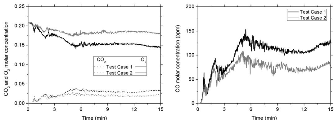
Figure 5: Time evolution of O<sub>2</sub> and CO<sub>2</sub> (left) and CO concentrations (right) in the middle of the kitchen, at a height of 1.6 m.
