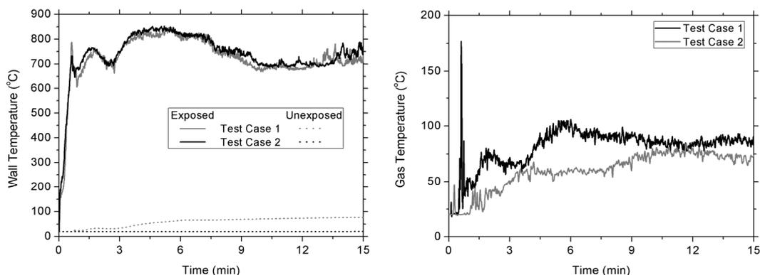
Figure 4. Temporal evolution of the surface temperature of the kitchen wall adjacent to the fire origin (left) and the gas temperature in the middle of the kitchen, at a height of 1.6 m (right).
