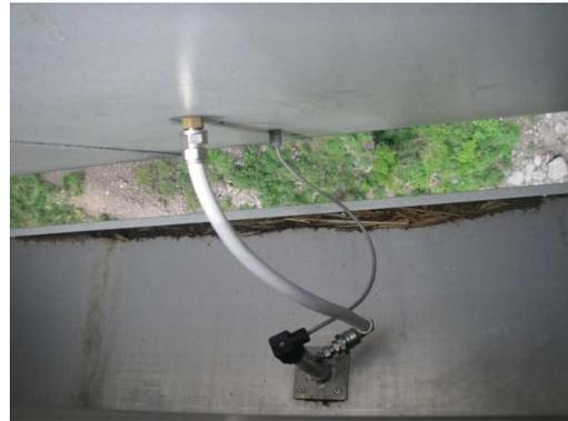
*Figure 1: Wind Pressure sensor*
