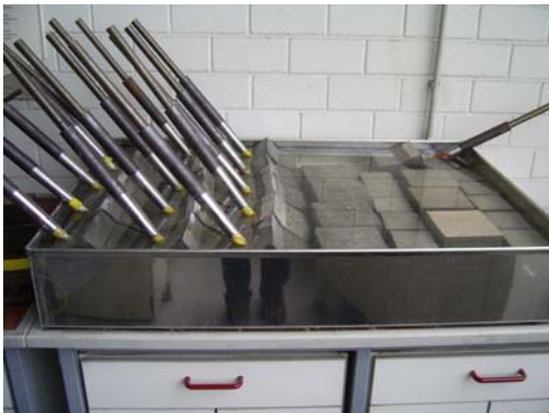
Figure 1: Curing of test specimen in water.
