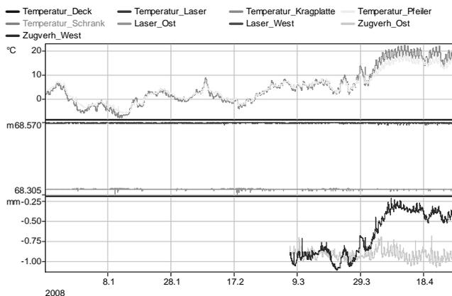
Figure 7. Results for temperature (top), arch distance (middle) and tendons (bottom)
