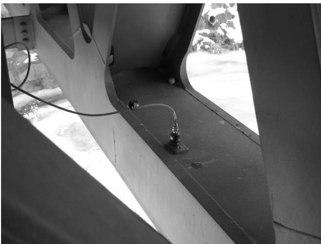
Figure 8. Acceleration Sensor on bridge girder
