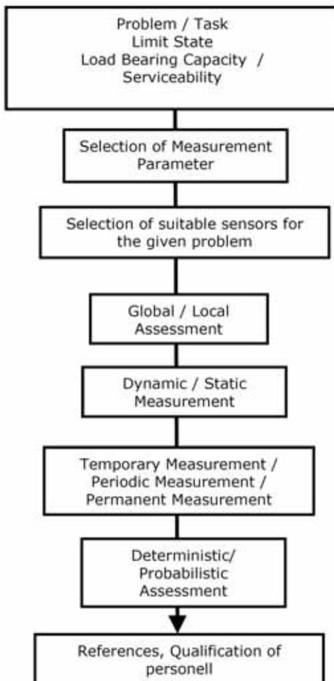
Figure 1. Flowchart of the Austrian monitoring guideline
