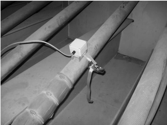
Figure 2. Acceleration sensor on stay cable
