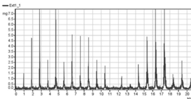
Figure 4. Typical frequency spectrum of one cable
