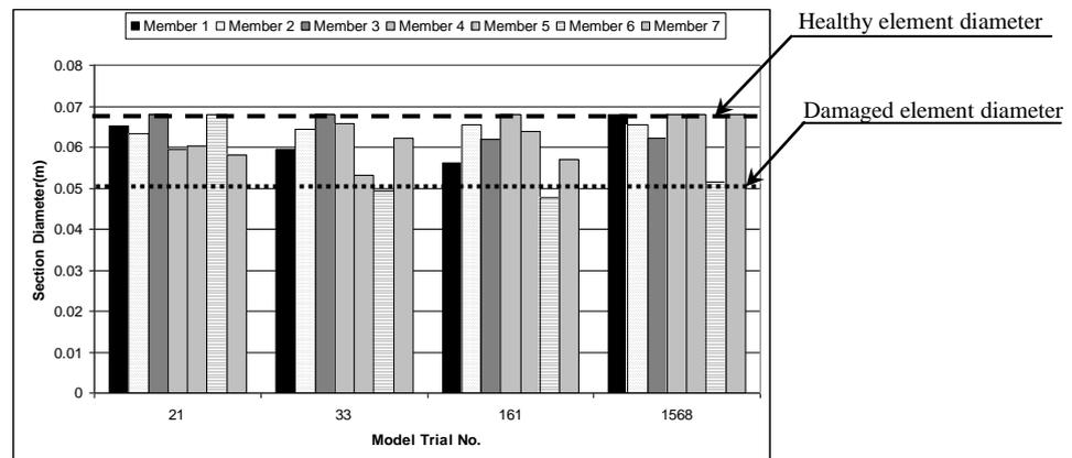
Figure 6 Snapshots of GA solution trials for the identified member diameters of the truss structure
