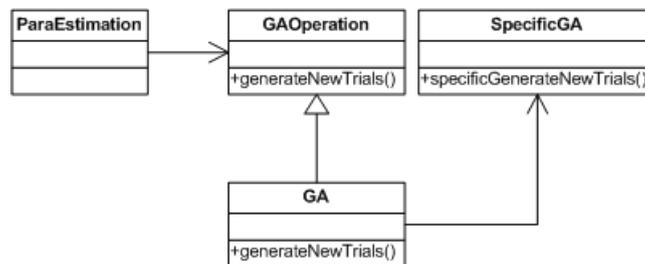
Figure 4 Object adapter pattern for GA
