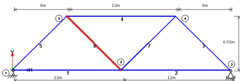
Figure5 Dimension of example truss structure
