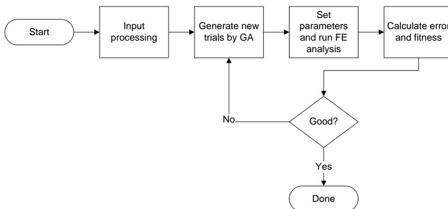
Figure 1 Data flow of finite element model updating method
