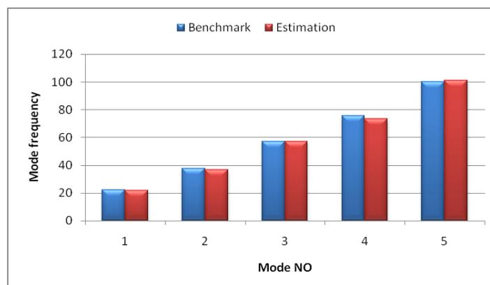
Figure 7 Comparison of mode frequencies between the FE model estimated and the observed benchmark
