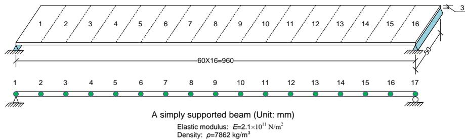
Figure 1. Simply supported beam model
