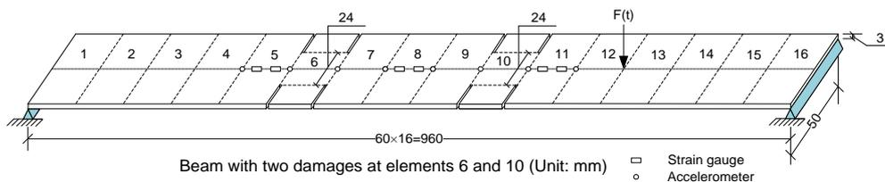
Figure 2. Damage scenarios and sensors placements
