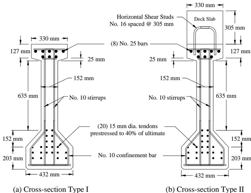
Figure 1. Cross-sectional configurations of MoDOT Type 4 experimental PC girders.
