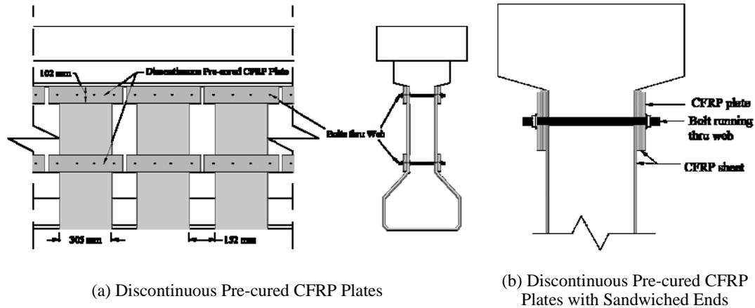
Figure 4. CFRP anchorage systems from experimental program.
