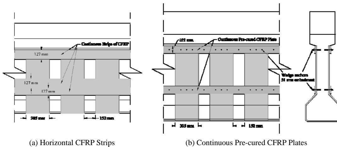
Figure 3. CFRP anchorage systems from experimental program.
