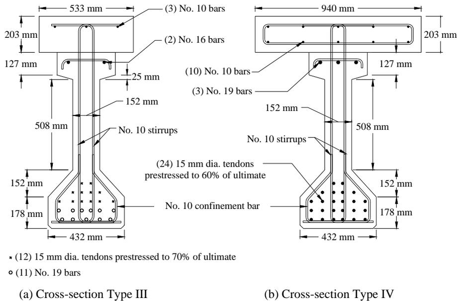
Figure 2. Cross-sectional configurations of MoDOT Type 3 experimental PC girders.
