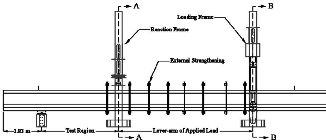
Figure 5. General test set-up for PC girders.
