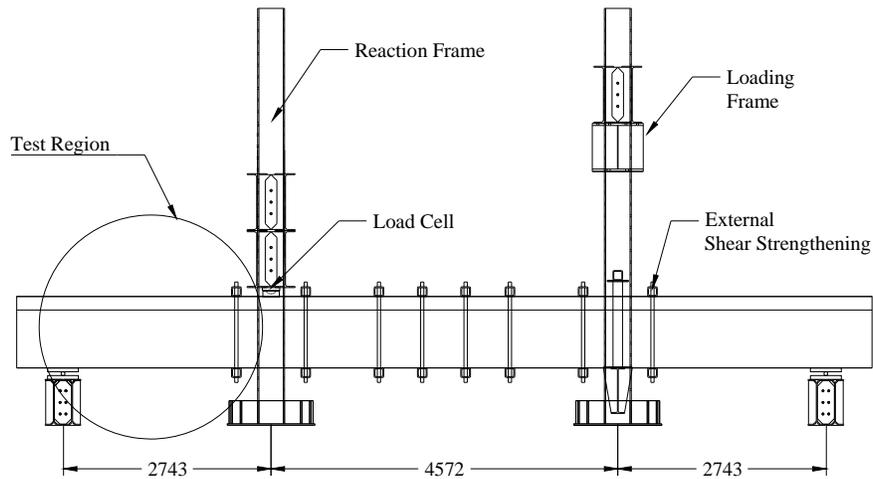
Figure 2. Details of test set-up (dimensions in mm).
