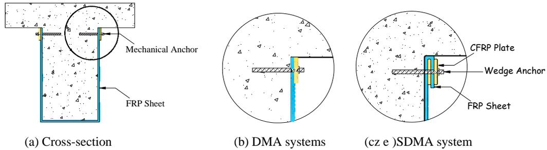
Figure 4. Details of mechanical anchorage system.
