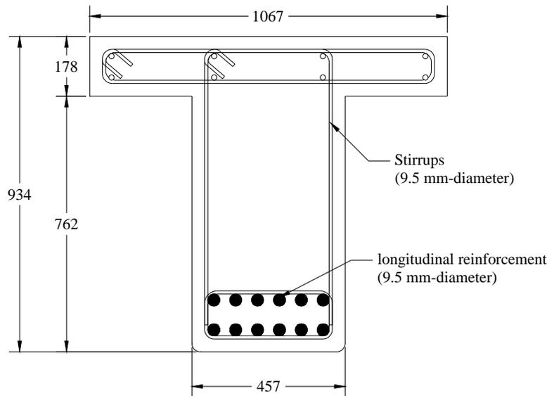
Figure 1. Cross section of the test beams used in this study (dimensions in mm).
