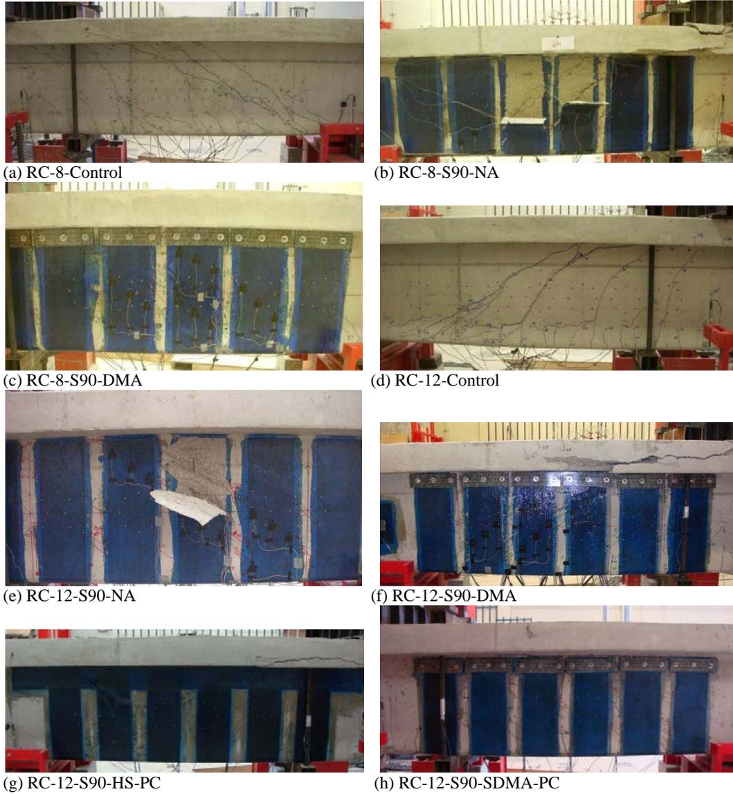
Figure 5. Failure Modes.
