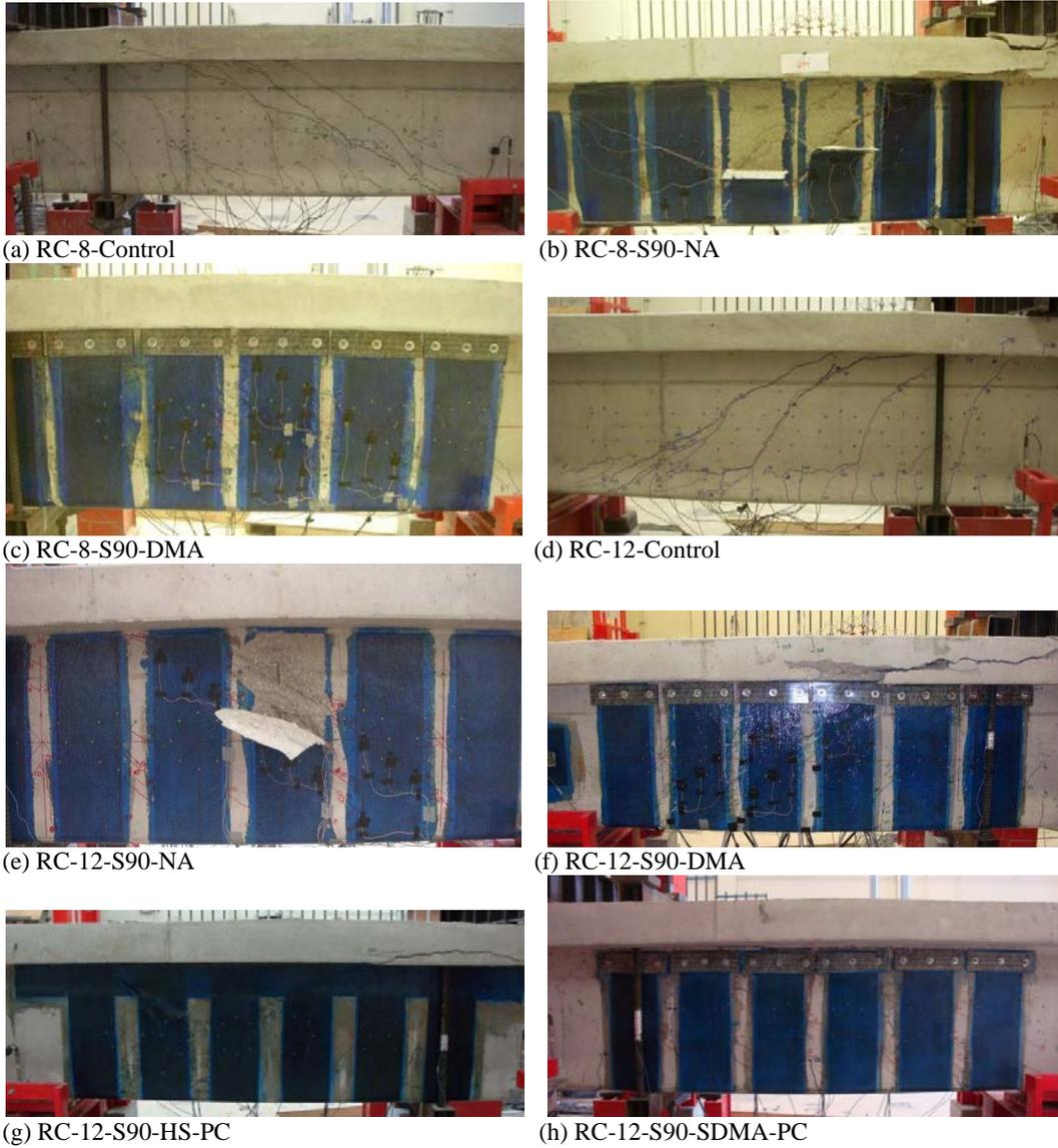
Figure 5. Failure Modes.
