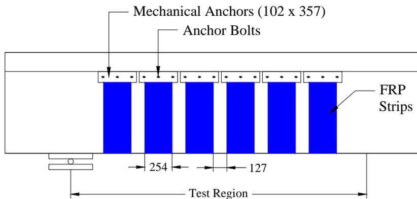
Figure 3. Configuration of externally bonded CFRP sheet strengthening with mechanical anchorage system (dimensions in mm).
