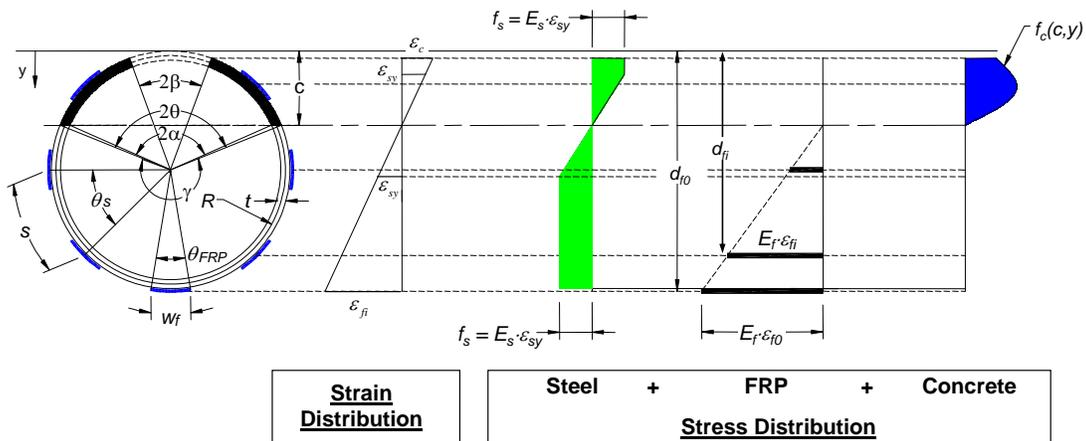
Figure 1. Stress-Strain Distribution (Opening in Compression)
