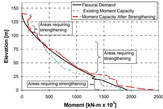
Figure 2. Demand vs. Capacity for Un-Strengthened and Strengthened Chimney
