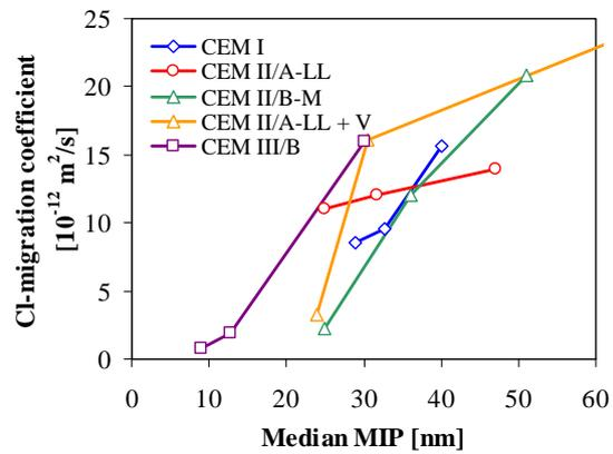
Figure 10: Chloride migration coefficient versus the median of the pore size distribution determined with MIP.
