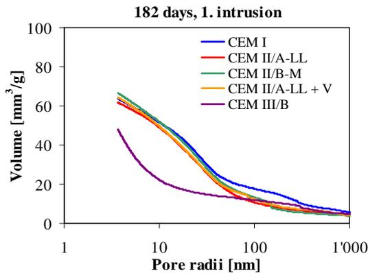
Figure 4: Total porosity and pore size distribution of mortar determined with MIP at an age of 182 days.
