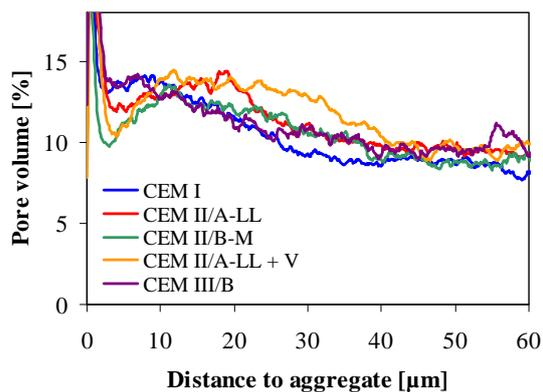
Figure 6: Pore volume in the different mortars as a function of the distance to the aggregates.
