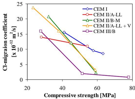
Figure 8: Chloride migration coefficient versus compressive strength.
