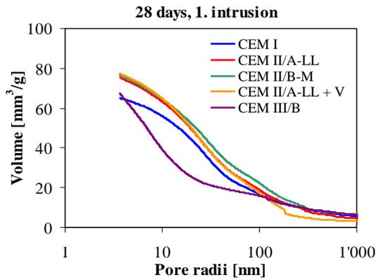
Figure 3: Total porosity and pore size distribution of mortar determined with MIP at an age of 28 days.
