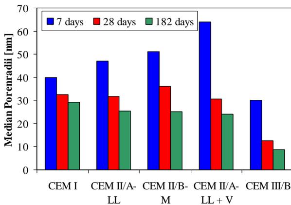
Figure 5: Median of the pore size distribution determined with MIP.
