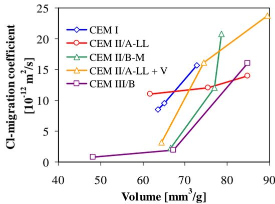
Figure 9: Chloride migration coefficient versus total porosity determined with MIP.
