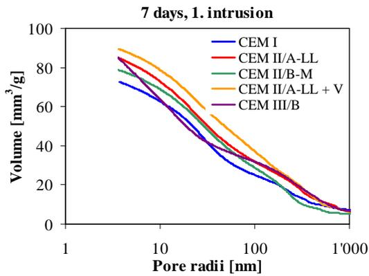
Figure 2: Total porosity and pore size distribution of mortar determined with MIP at an age of 7 days.
