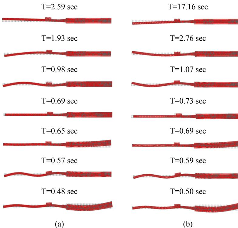
Figure 4. Modal deformed shapes and periods for first section: (a) fixed restraint; (b) hinge restraint.
