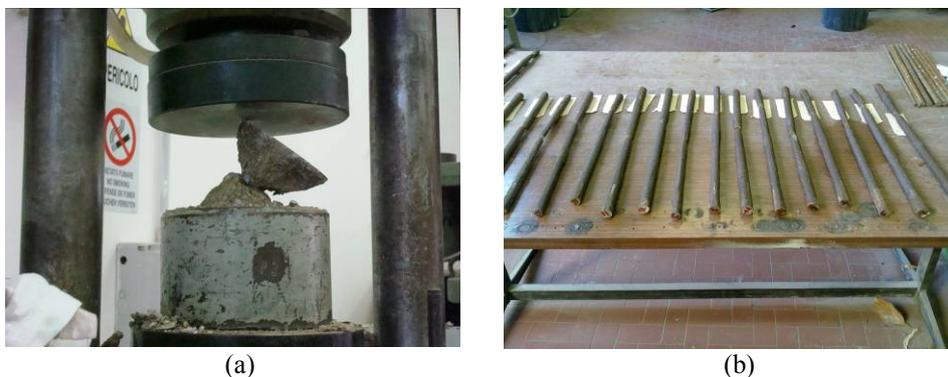
Figure 3. Destructive Material characterizations, failure of: (a) concrete specimens; (b) steel specimens
