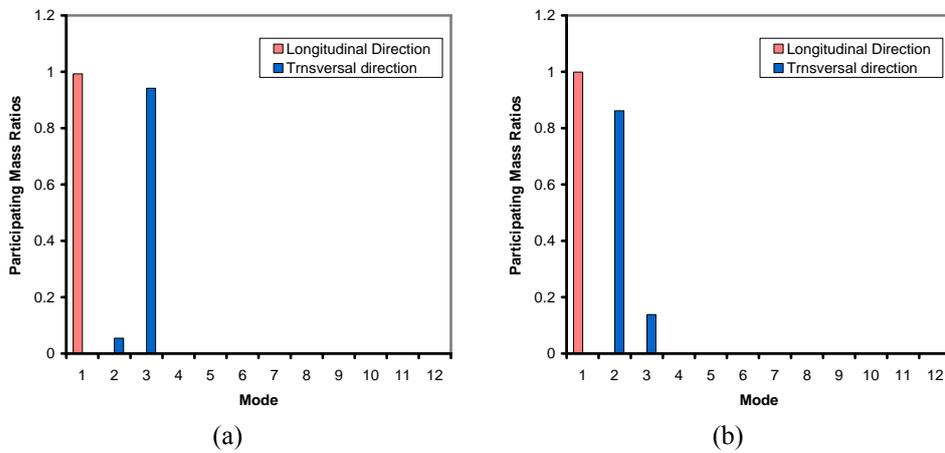
Figure 7. Participating mass ratios for second section: (a) fixed restraint; (b) hinge restraint.
