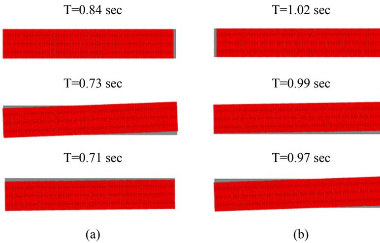
Figure 6. Modal deformed shapes and periods for second section: (a) fixed restraint; (b) hinge restraint.
