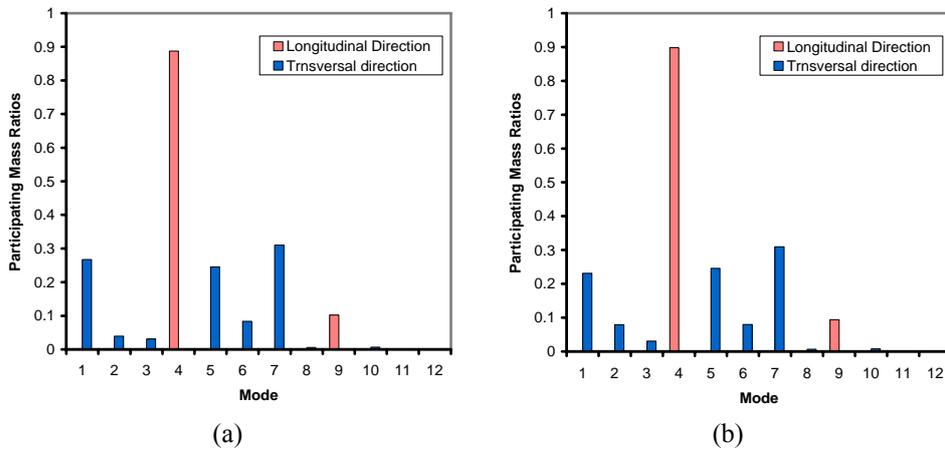
Figure 5. Participating mass ratios for first section: (a) fixed restraint; (b) hinge restraint.
