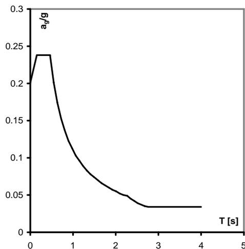
Figure 8. Response spectrum for seismic analyses.
