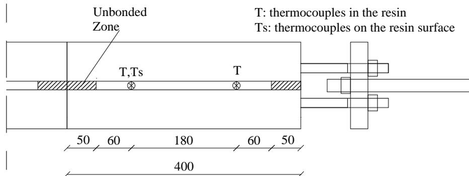
Figure 3. Thermocouples location within the test specimen.
