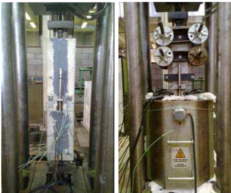
Figure 2. Specimen in the tensile machine without and with oven
