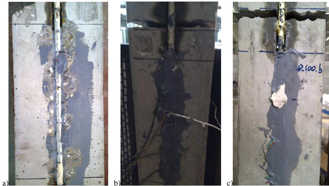
Figure 4. Failure modes a) debonding with splitting of the resin, b) debonding at epoxy/concrete interface, c) debonding with pull-out of the bar.
