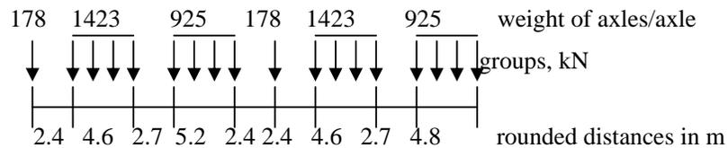
Figure 5. Cooper E80 design load with a total weight of 5,053 kN and a base length of 33.2 m.
