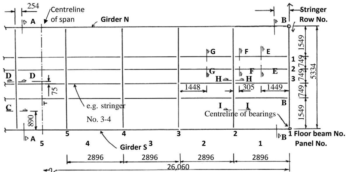
Figure 2. Partial plan of the bridge showing instrumented sections (all dimensions in mm)
