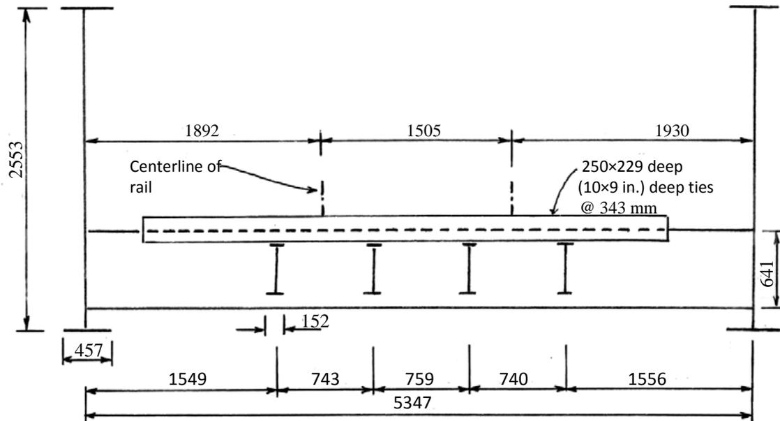
Figure 1. Cross-section of the railway bridge (all dimensions in mm)
