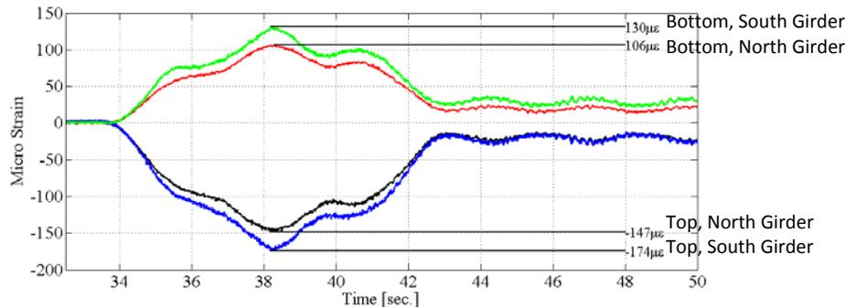
Figure 7. Observed strains in girders near mid-span due to the 1<sup>st</sup> train
