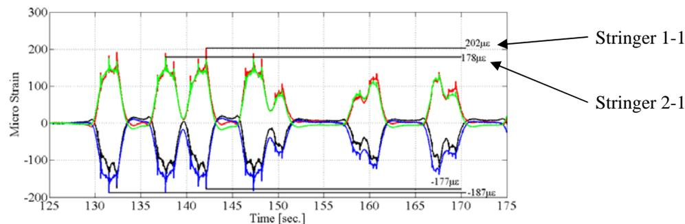
Figure 6. Strains in stringers due to the 1<sup>st</sup> train
