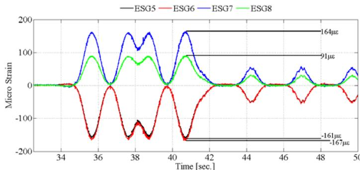
Figure 8. Strains due to the 1<sup>st</sup> train in floor beam No. 6
