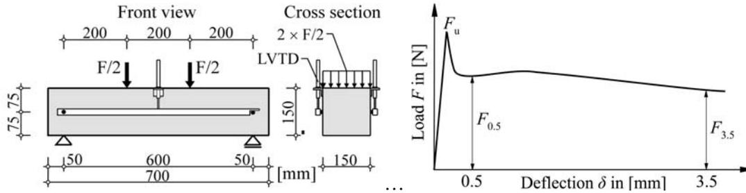
Figure 3. Test set-up and analysis of the four-point bending test
