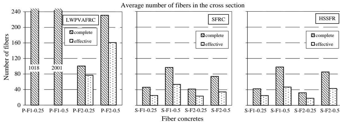
Figure 5. Average number of fibers in the cross section of the tested beams
