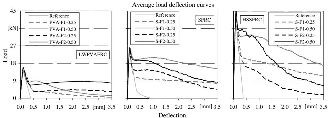
Figure 4. Average load deflection curves of different fiber concretes
