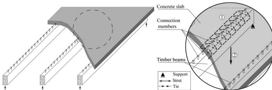
Figure 1. Principle structure of a TCC ceiling (left), loading of the concrete slab (right)
