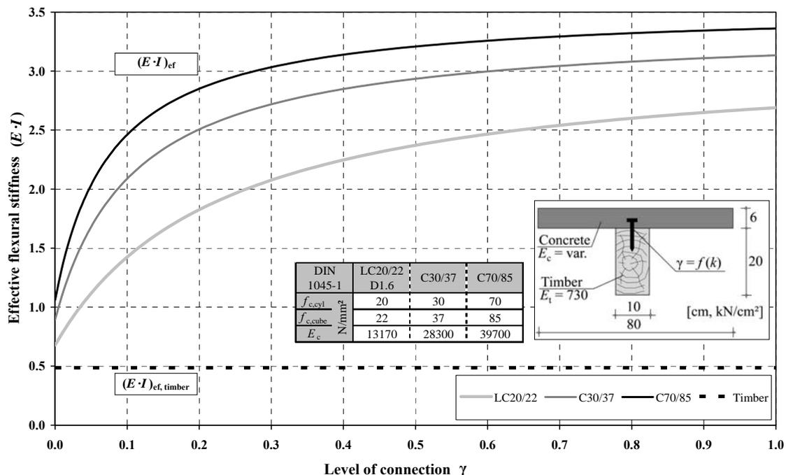
Figure 2. Influence of the modulus of elasticity on the stiffness of a TCC construction
