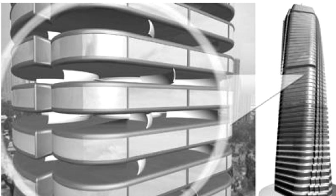
Figure 3. Vertical axis turbines located between floors all along the tower height (Fisher 2008).
