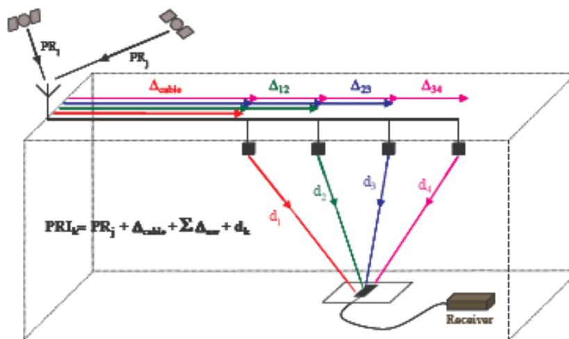
Figure 5. Basic principle of inside amplified GPS receiver unit.
