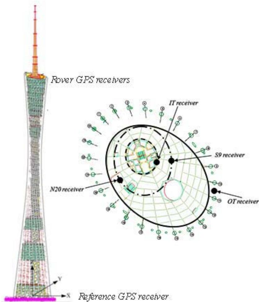
Figure 4. Location of the measurement points for GPS sensors (vertical and plan view). The figure also shows the oval shape at the top plane section (450m height) in which the numbers 9 and 20 at the edge indicates the position of *S9* and *N20* receivers. Three GPS rover sensors are placed at the top level and the reference one at the base.
