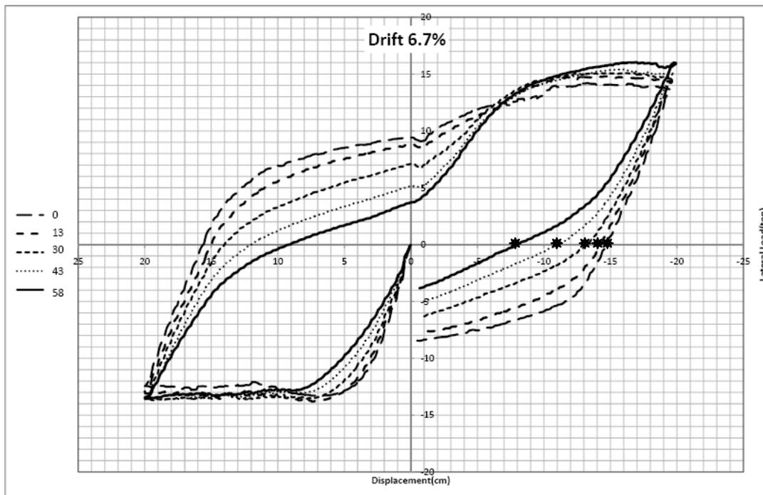
Fig. 4 . Hysteresis curve of shear force versus displacement for models
