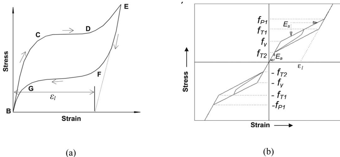
Fig. 1. (a) Typical axial stress-strain diagram of SMA, (b) 1D model of SMA incorporated in FE packages
