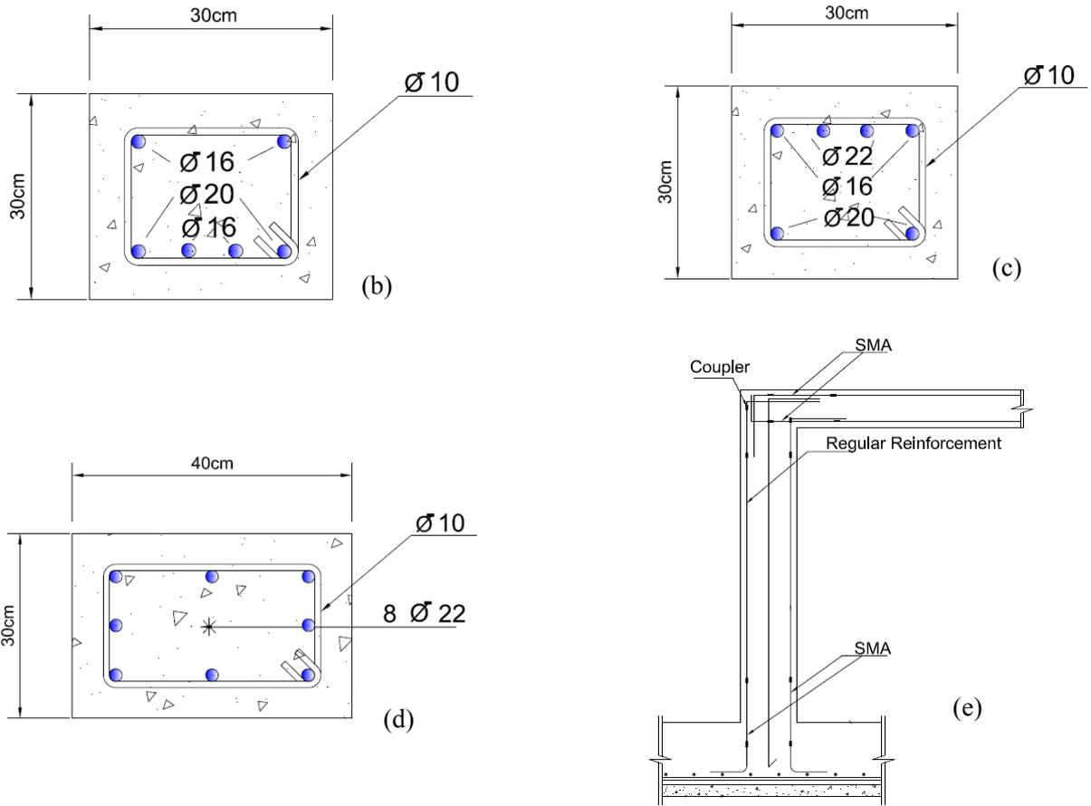
Fig. 2 (a) designed frame under ACI considerations (b) middle section of beam (c) section of beam near connection (d) column section (e) arrangement of SMA in the frame
