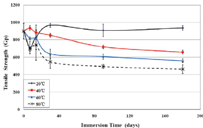
Figure 5. Variation of the tensile strength of BFRP rebars as a function of immersion time in distilled water at different temperatures.
