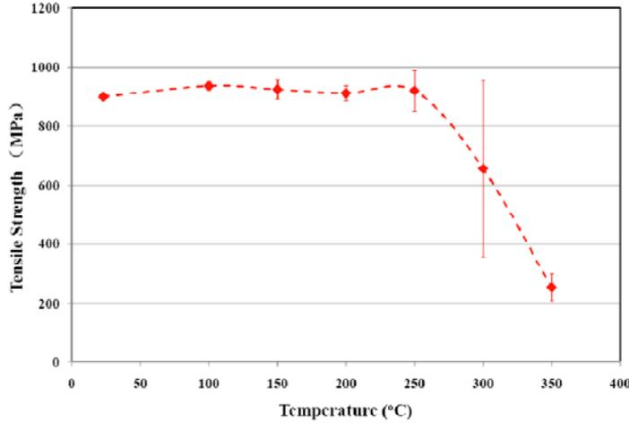
Figure 2. Tensile strength of BFRP rebar at various temperatures.
