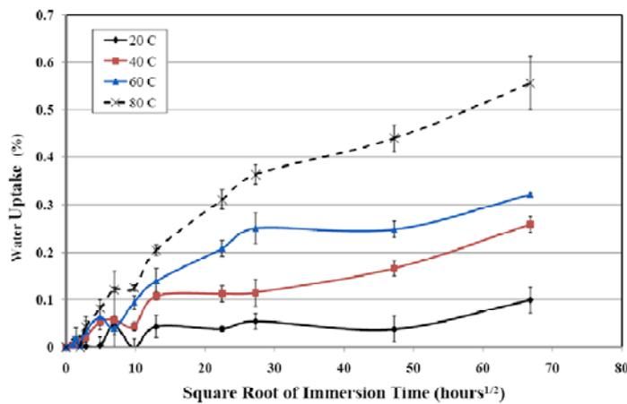
Figure 4. Water uptake of BFRP rebars of 30 mm in length and 8 mm in diameter immersed in distilled water.
