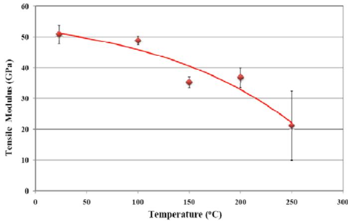
Figure 3. Tensile modulus of BFRP rebar at various temperatures.
