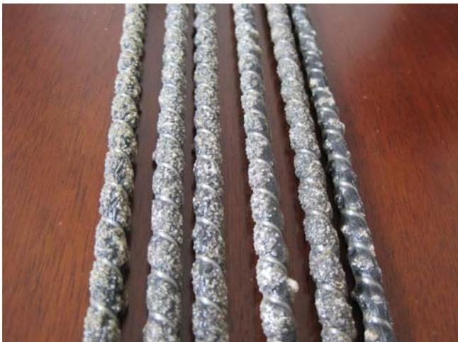
Figure 1. Photograph of BFRP rebars with a nominal diameter of 8 mm.
