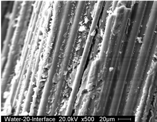
Figure 6. Fractography picture of BFRP rebars (23°C water immersion for 6-month) after tension test.
