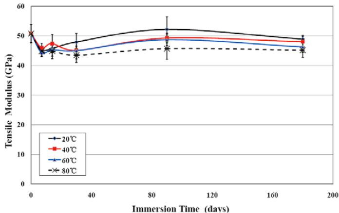
Figure 8. Variation of the tensile modulus of BFRP rebars as a function of immersion time in distilled water at different temperatures.
