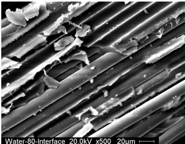
Figure 7. Fractography picture of BFRP rebars (80°C water immersion for 6-month) after tension test.
