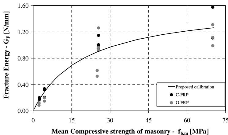
Figure 5. Fracture energy  $G_F$  vs. mean compressive strength of masonry: proposed rational relationship
