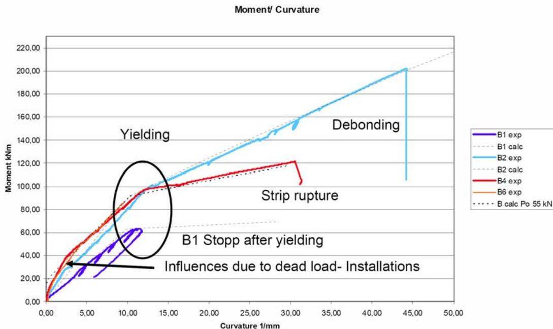
Figure 10: Moment Curvature diagram
