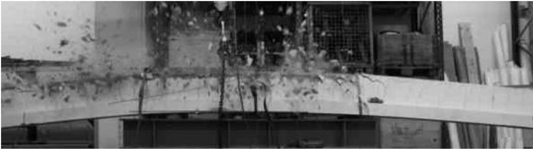
Figure 9: Debonding of concrete cover of beam 2, strengthened with 3 untensioned strips.
