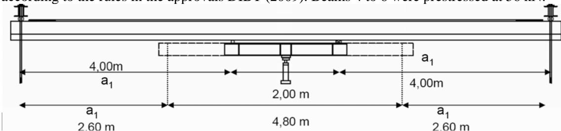
Figure 7: 4 point bending test
