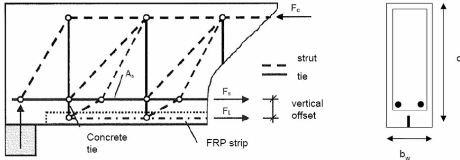
Figure 1: Extended strut and tie model for strengthened cross section Schäfer (1996).
