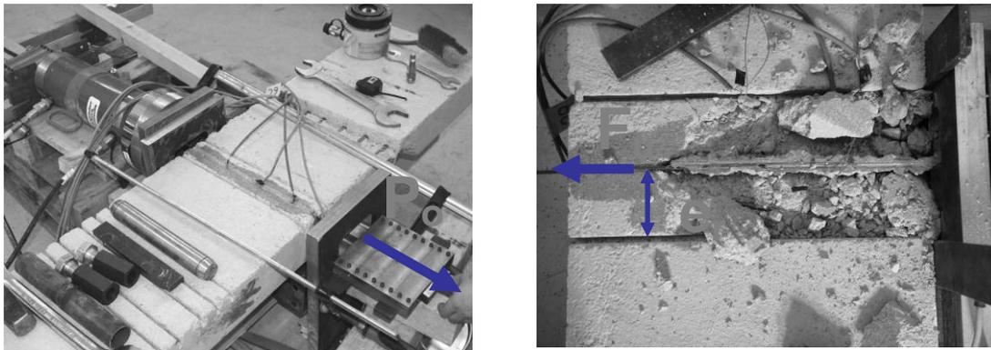
Figure 4: Test Set up pull out test left  $e_r = 36$  mm, concrete failure right for  $e_r = 75$  mm,
