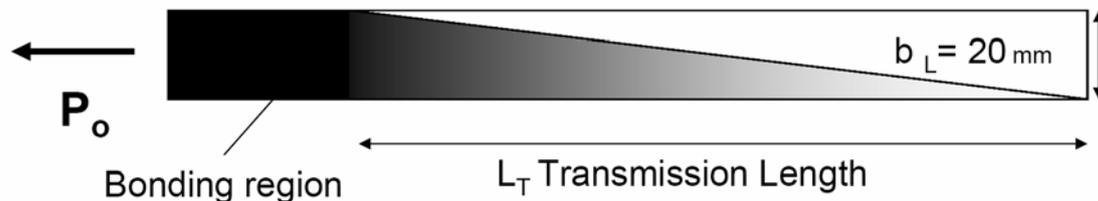
Figure 2: Transmission bonding of the strip
