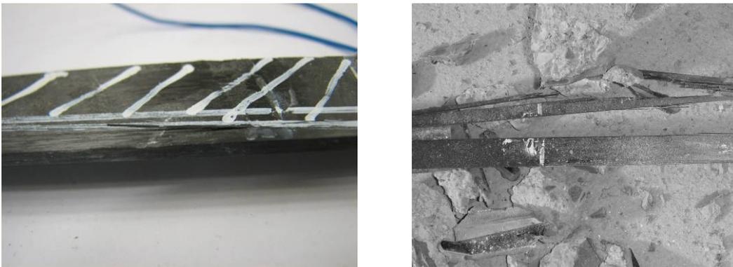
Figure 5: FRP failure: left specimen 4  $P_0 = 43$  kN right specimen 6  $P_0 = 53$  kN
