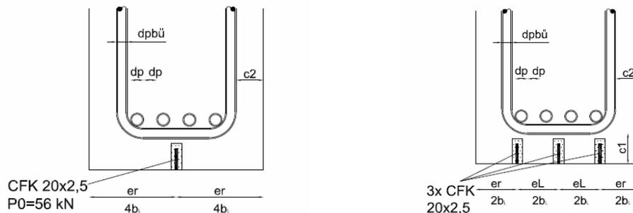
Figure 6: Strip application left the prestressed and right NSM application.
