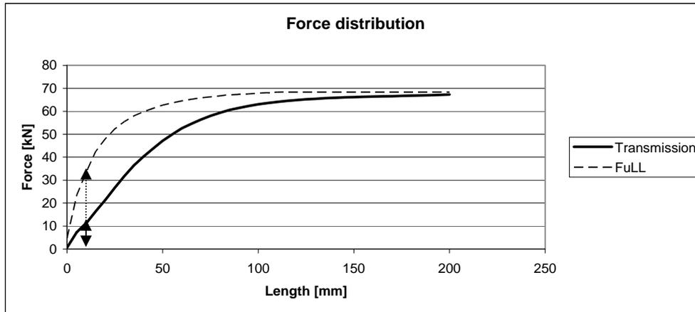
Figure 3: Load and stress distribution of FE - analysis
