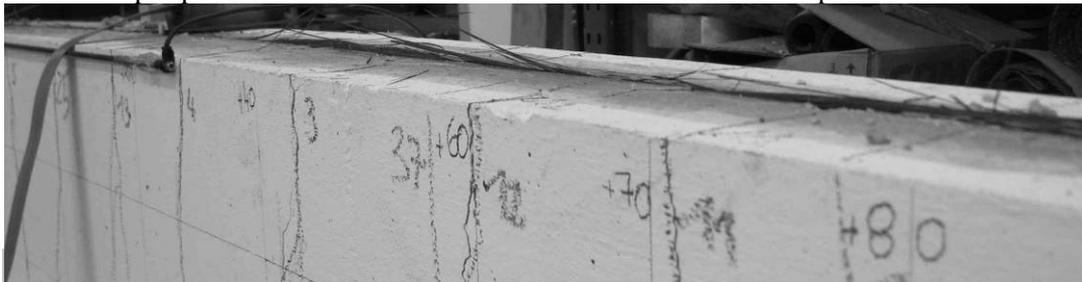
Figure 8: Strip rupture at maximum load for Beam 5
