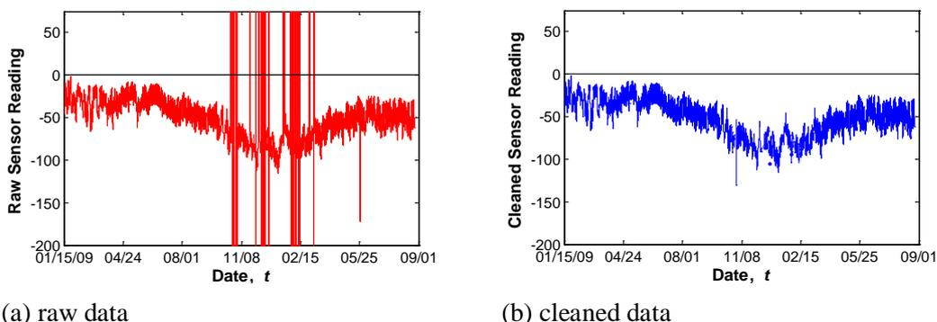
Figure 5. Removal of outliers from raw data (sensor #22 – VW on G1 (bottom) at Bent 24 in Span 23).
