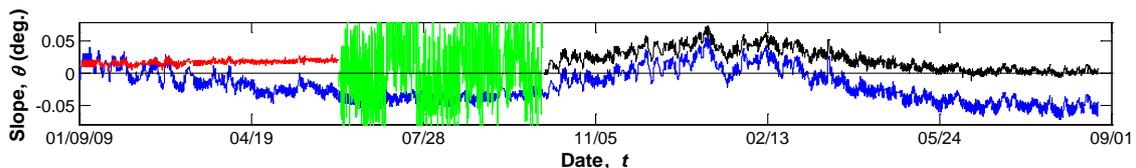
Figure 7. Joined data record for tiltmeter (TM) at G1 in Span 24.
