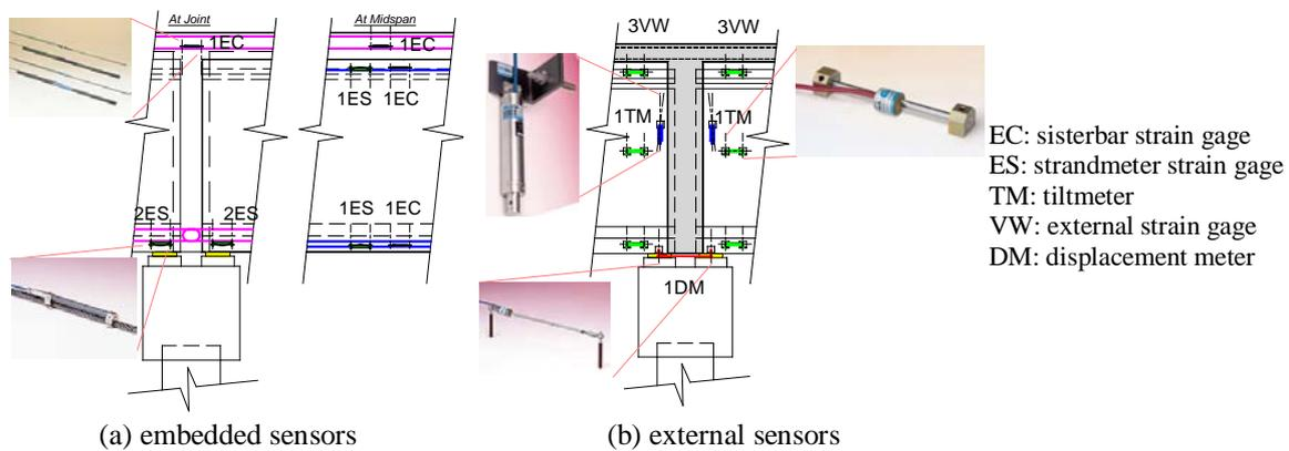
Figure 3. Layout of employed sensors.
