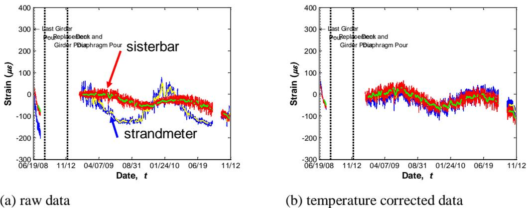
Figure 6. Temperature correction of sensors #88(ES) and #94(EC) in G3 (bottom) at Midspan 24).
