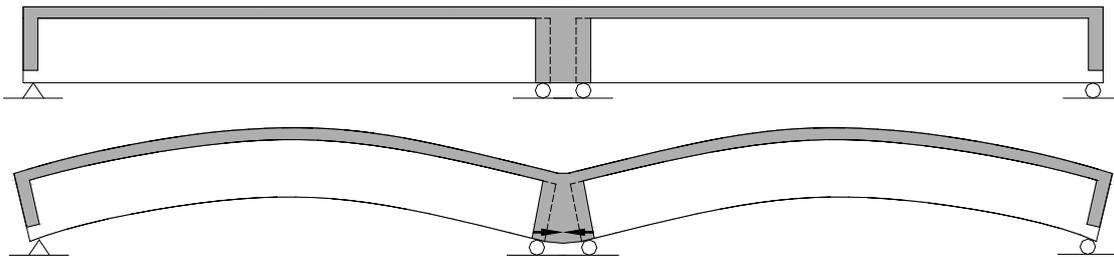
Figure 1. Development of positive moment in bridge connections with continuity diaphragm.
