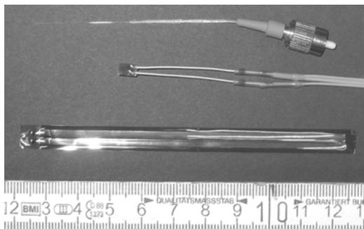
Figure 2. Optical fiber with link and different strain gauges.
