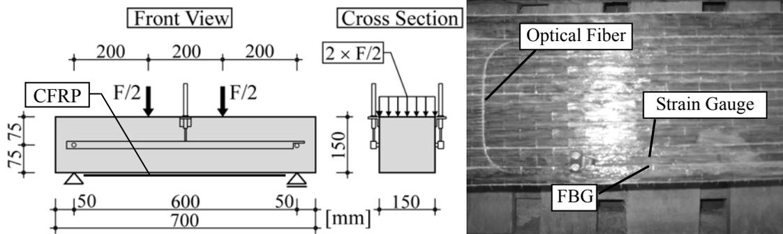
Figure 4. Test set-up of the four point bending test and arrangement of the optical fiber measurement system (Test program 1).
