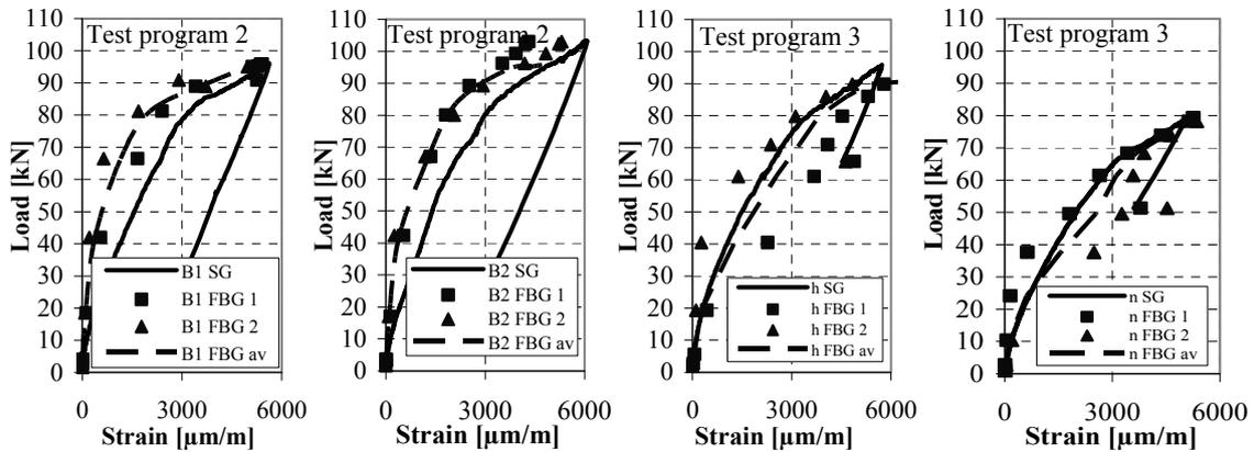
Figure 6. Load strain curves of strain gauge and FBG by use of concrete C60/75 (h) (Test program 2 and 3) and C30/37 (n) (Test program 3).
