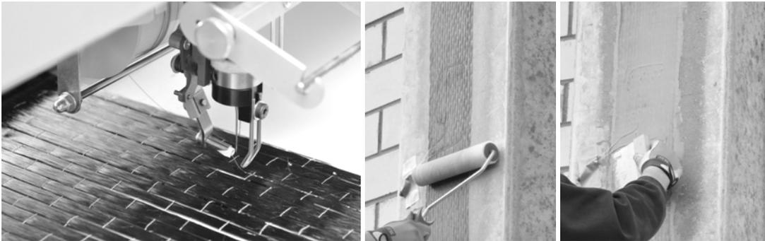
Figure 3. Production of sensor based CFRP (First: embroider of optical fiber; Second: lamination by hand at building site).
