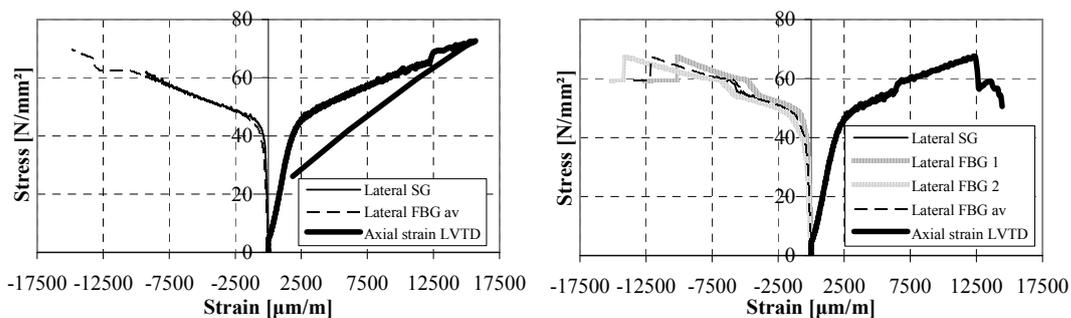
Figure 7. Stress strain curves of strain gauge (SG) and FBG average (FBG av) of column 1 and 2.
