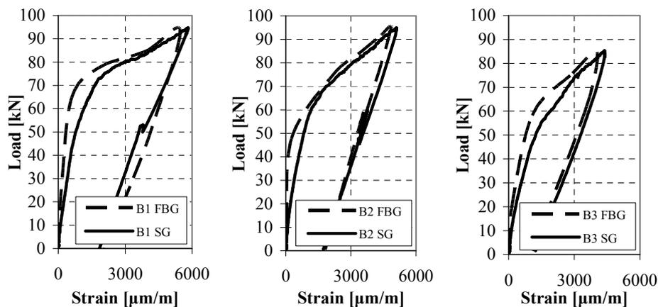
Figure 5. Load strain curves of strain gauge (SG) und Fiber Bragg Grating (FBG) (Test program 1).
