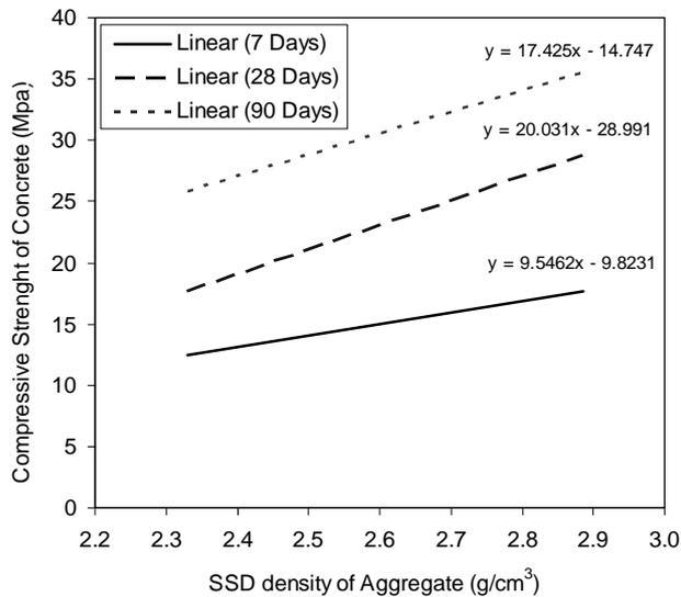
Figure 2. Effect of density of aggregates on compressive strength of concrete.
