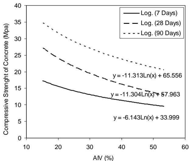
Figure 7. The relationship between AIV of aggregate and compressive strength of concrete.
