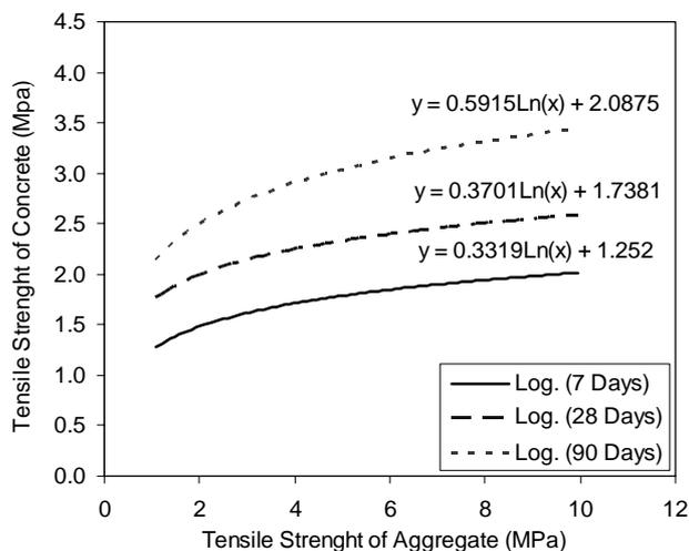
Figure 5. The relationship between tensile strength of aggregate and tensile strength of concrete.
