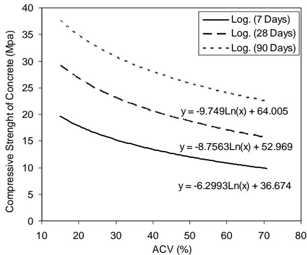
Figure 6. The relationship between ACV of aggregate and compressive strength of concrete.
