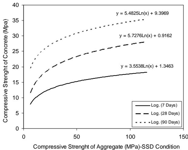
Figure 4. The relationship between UCS of aggregate and compressive strength of concrete.
