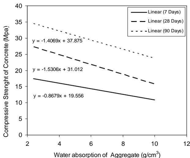
Figure 1. The relationship between water absorption of aggregates and compressive strength of concrete.
