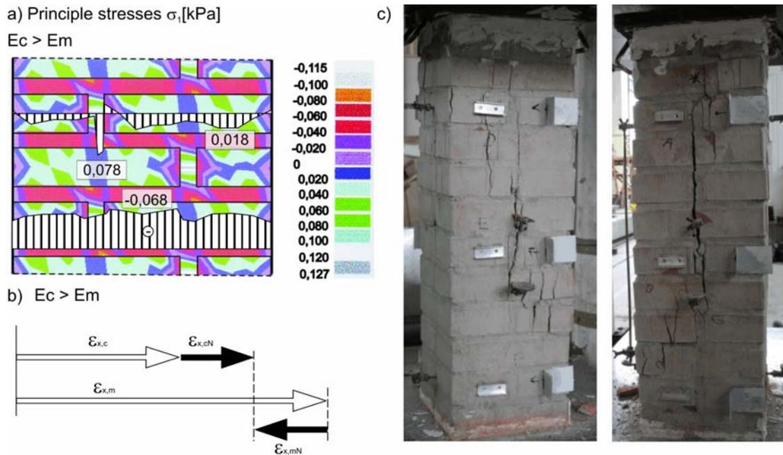
Fig. 6 a) The pattern of principal stresses  $\sigma_1$  in a compressed masonry pillar (450 mm in thickness); b) Mechanism of mutual co-action of masonry units and mortar; c) Characteristic failure of a non-strengthened masonry pillar at the ultimate load
