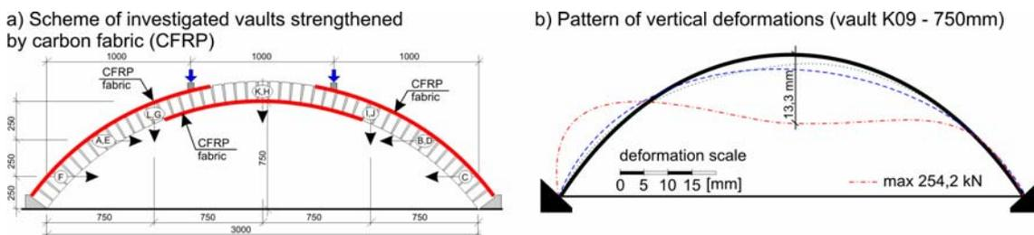
Fig. 3 a) Scheme of investigated vaults strengthened by carbon fabric; b) The pattern of vertical deformations of a vault with a vertical rise of 0.75 m (K09) strengthened by carbon fabric (prominent non-symmetry of the deformation line of a symmetrical vault, symmetrically loaded);
