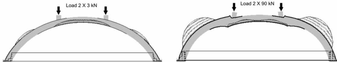
b) Ultimate load-bearing capacities of vaults
