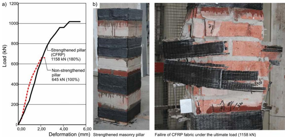
Fig. 7 a) Experimentally determined working diagrams of non-strengthened masonry pillars and pillars strengthened by carbon fabric; b) Strengthening of masonry pillars by wrapping them in carbon fabric and characteristic failure of a strengthened pillar
