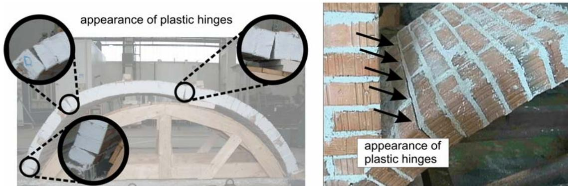
Fig. 1 Characteristic failures of non-strengthened masonry barrel vaults by tensile cracks
