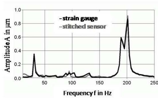
Figure 3: Diagram of free vibration decay test      Figure 4: Signal of embroidered sensor and strain gauge
