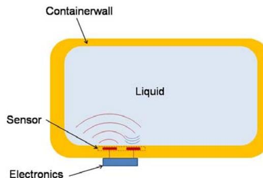
Figure 3: Functional principle of a capacitive fill level measurement system
