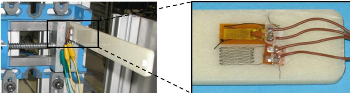
Figure 2: Beam arrangement to compare embroidered sensor with regular strain gauge
