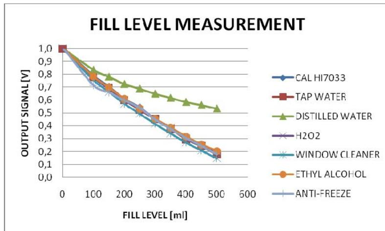
Figure 6: Fill level measurements of different liquids
