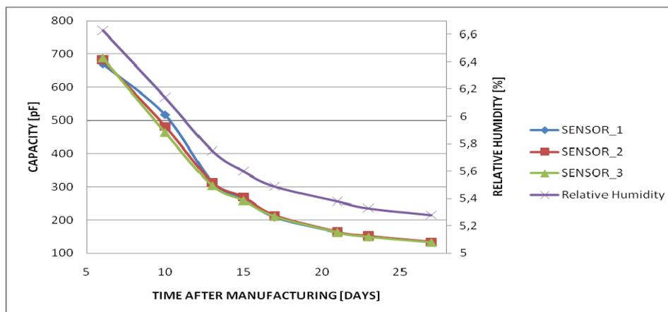
Figure 7: Correlation between sensor signal and relative humidity
