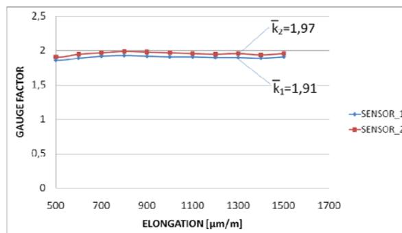
Figure 6: Gauge factor measurement
