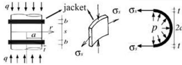
Figure 1: Cylinder loaded by axial pressure and confined by active lateral pressure [Mortazavi et al (2003)].
