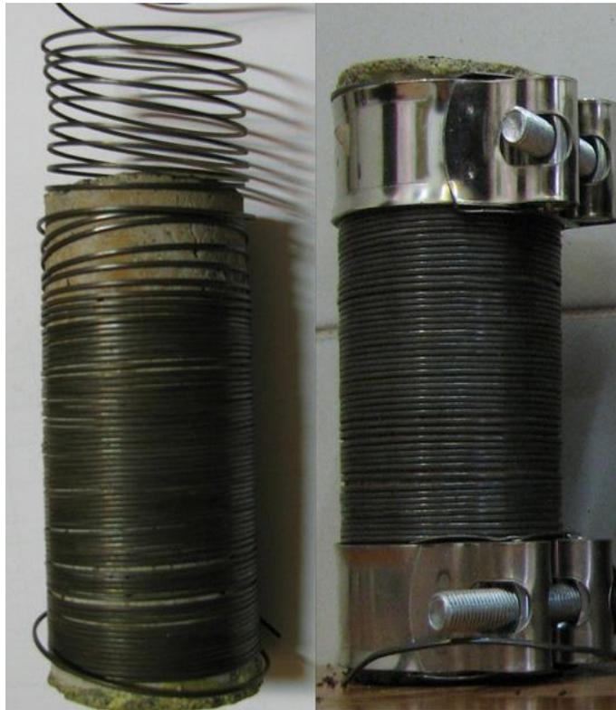
Figure 2: SMA wire wrapped around the concrete cores and anchored with steel clamps
