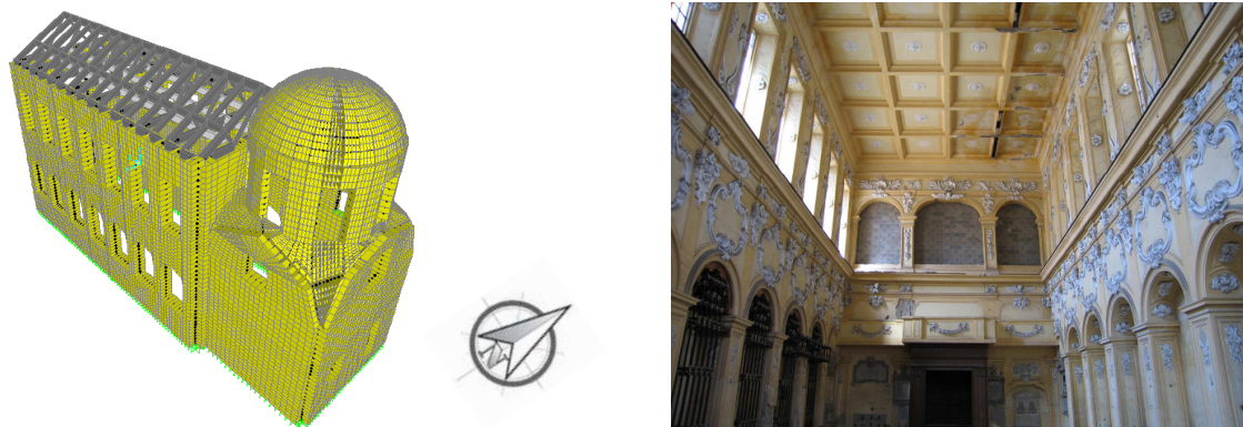
Figure 1. Naples, church of St. Maria del Popolo. Perspective view of the 3D FE model of the church, and inner view of the roof.
