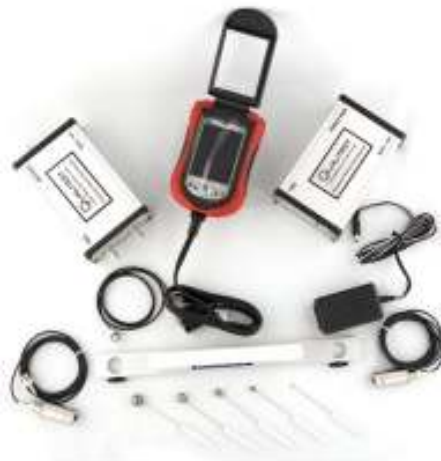
Figure 5 Portable Impact-Echo System Field Kit
