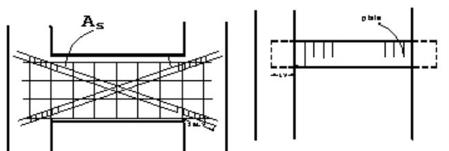
Figure 5.Concrete link beam with diagonal rebar and steel link beam with plate
