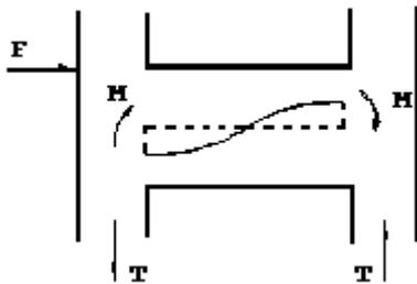
Figure 4.Forces in couple shear wall with lateral force
