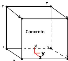
Figure 6. Eight-node element used in numerical model
