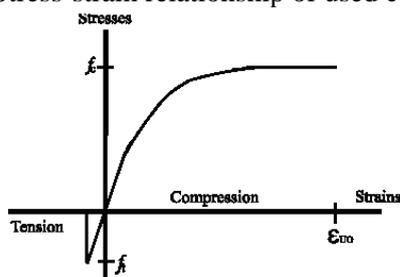
Figure 7. Concrete stress-strain curve used in finite element program
