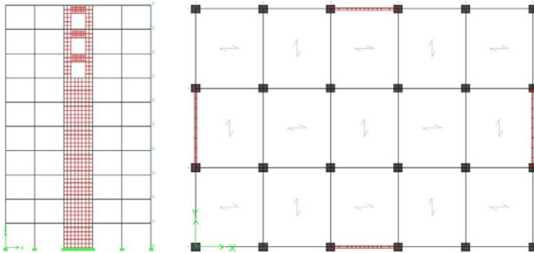
Figure 3. Plan and elevation of numerical model of 10 story reinforced concrete building
