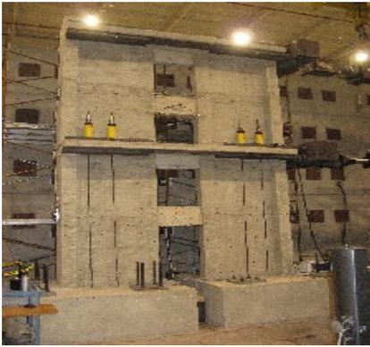
Figure 1. Coupled shear wall with concrete link beam
