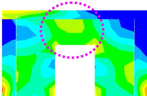
Figure 9. Stress in steel link beam (SSW)
