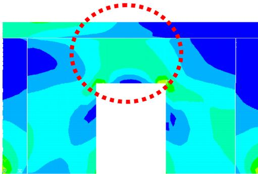
Figure 8. Stress in concrete link beam (CSW)
