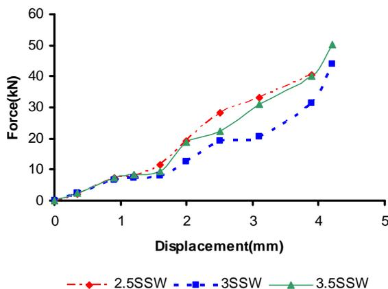
Figure12. Load- displacement curve of composite models
