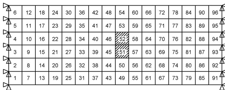
Figure 10: location of damaged elements
