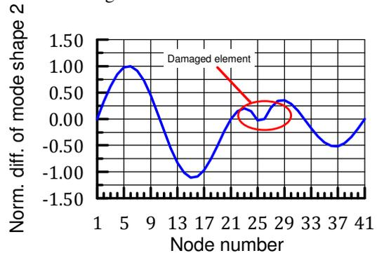
Figure 9: Normalized difference of mode shape 2 between intact and damaged beam
