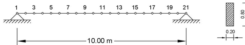
Figure 3: single span beam dimensions
