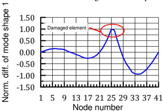
Figure 8: Normalized difference of mode shape 1 between intact and damaged beam
