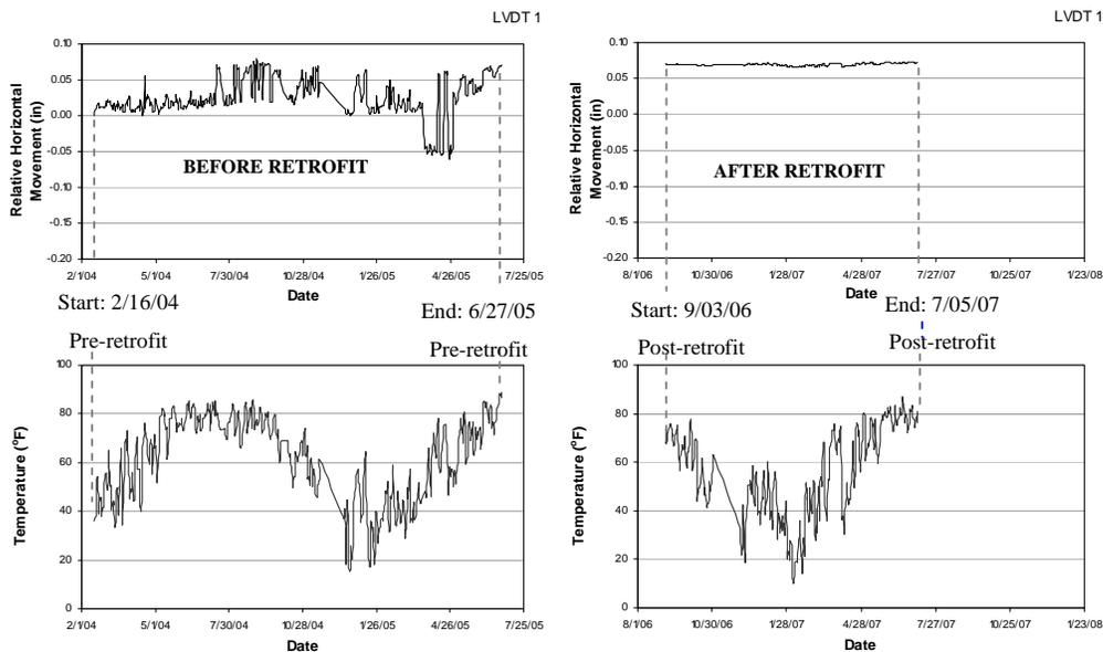
Figure 3. Relative horizontal movement measured at Beam 6 in Span 117.
