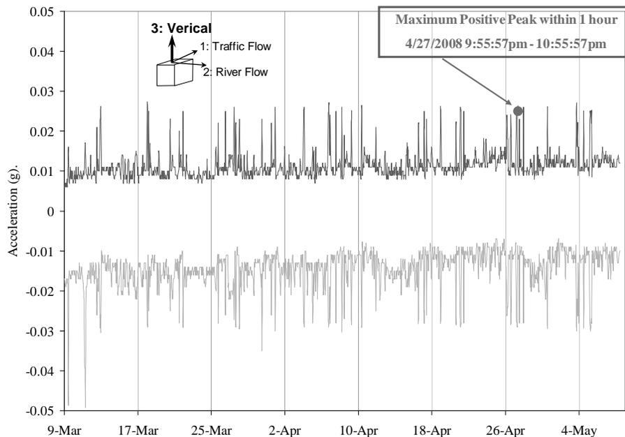
Figure 7. Maximum hourly vertical acceleration data at Pier D.
