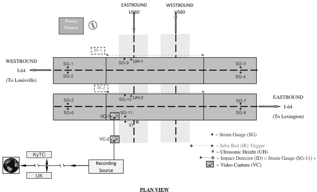
Figure 5. Gauge layout of I-64 Bridge over US60.
